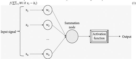
Fig.2. depicts the construction of a BP neural network. Adopted from hindwai. (Niu et al.)
