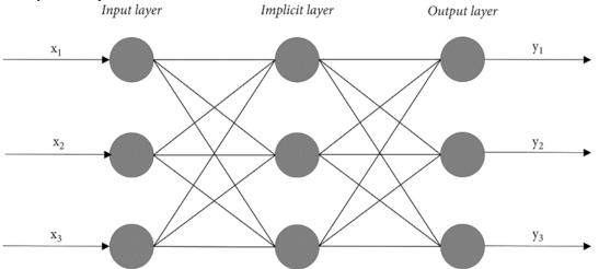
Fig.1. The algorithmic structure of a BP neural network Adopted from (Niu et al.)
