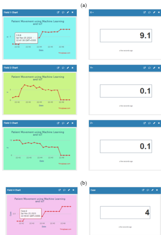
Figure 14: System results screen for the ThingSpeak website: a) Values of the three axes, b) Case number
