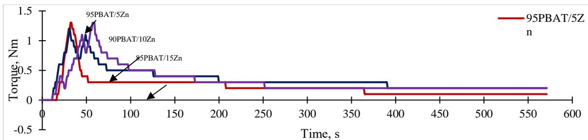
**Fig. 1:** Torque evolution curves for different composite compositions without PS (PBAT/Zn)
