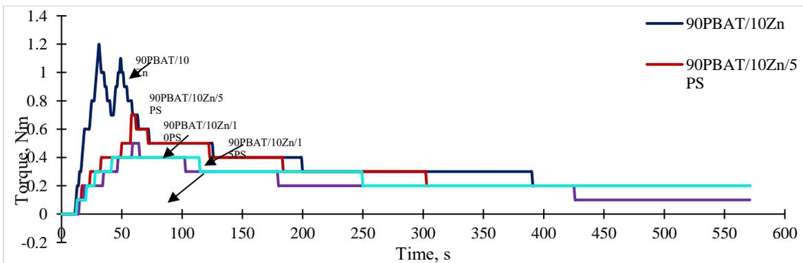
**Fig. 2:** Torque evolution curves for different composite compositions with PS (PBAT/Zn/PS)
