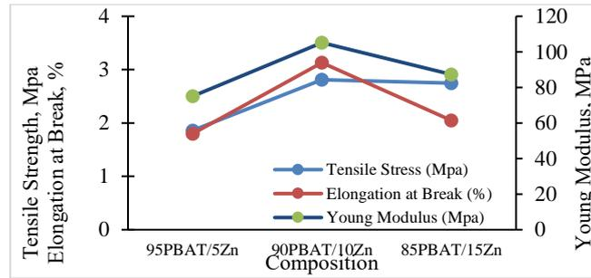
Fig. 5: The tensile strength (MPa), elongation at break (%) and young’s modulus (MPa) of PBAT/ZN blend
