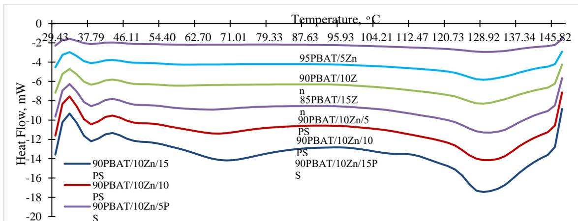
**Fig. 3:** DSC curves obtained for PBAT/Zn and PBAT/Zn/PS composite blends
