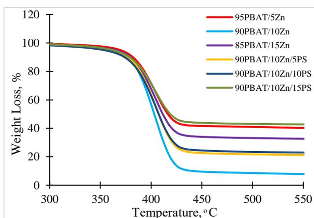
**Fig. 4:** TGA curves of PBAT/Zn and PBAT/Zn/PS blends
