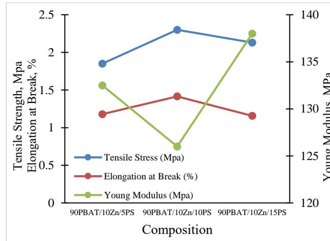
Fig. 6: The tensile strength (MPa), elongation at break (%) and young’s modulus (MPa) of PBAT/ZN/PS composites
