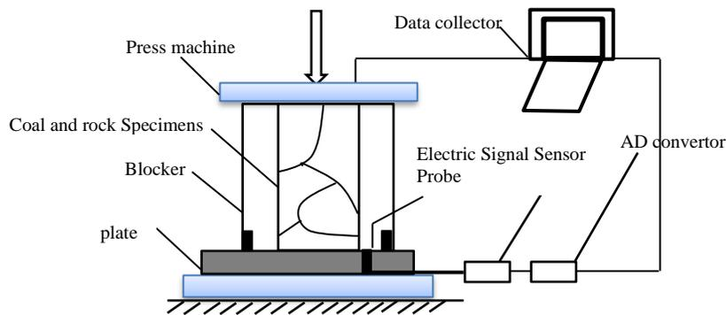
**Figure 3.1 (b) Diagrammatic Representation of the Coal Lithology Influence System on the Electrical Signal**
