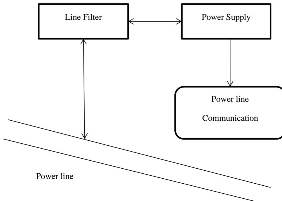
**Figure 1.1. Alternating mode power source for Power Line Transmission**
