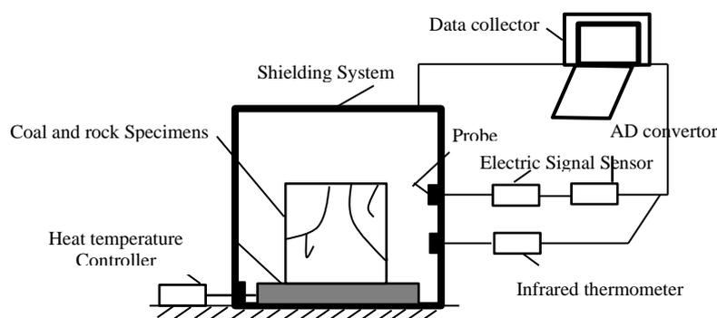
**Figure 3.1 (a). Diagrammatic Representation of How the Temperature of the Coal and Rock Affects the Electrical Signal**
