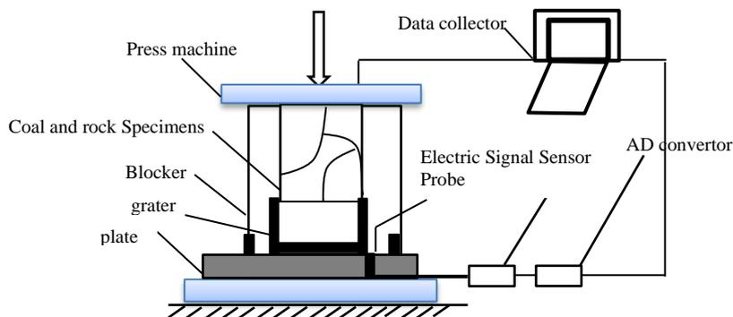
**Figure 3.1 (c) Diagrammatic Representation of the Coal-Rock Friction Influence System on the Electrical Signal**
