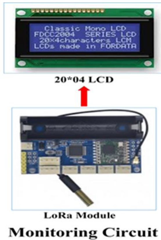
Figure 10: The receiving and monitoring circuit block diagram.
