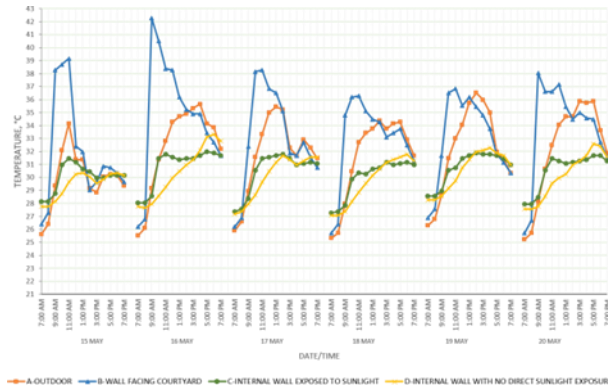
Fig.11. Indoor and Outdoor Temperature of Hakka Village.
