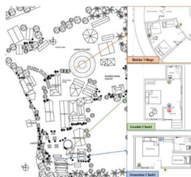
Fig 2. The Location of the Data Logger.
