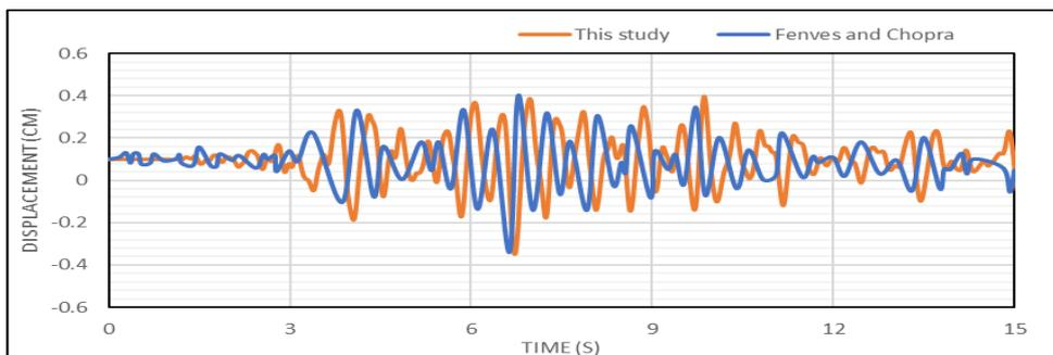
Figure 14 Heel Vertical Displacement (Nodal Point 3)
