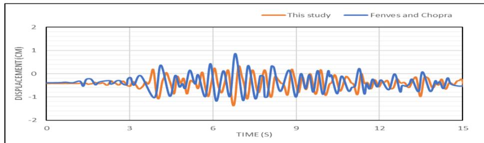
Figure 12 Crest Vertical Displacement (Nodal Point 8)
