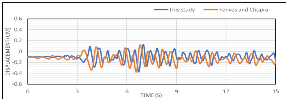
Figure 15 Toe Horizontal Displacement (Nodal Point 6)
