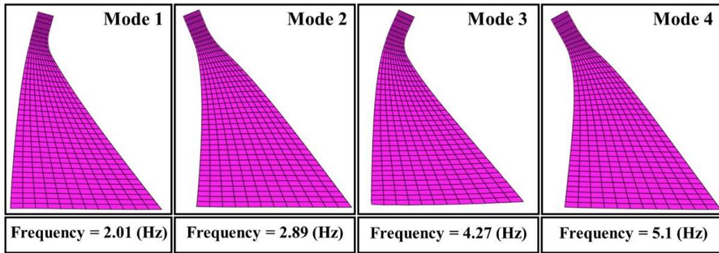
Figure 6 The Abaqus Model, Featuring a Flexible Foundation and a Full Water Tank, Exhibits its Initial Four Natural Frequencies.
