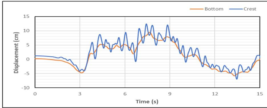
Figure 9 Temporal Variation of Displacement for the Heel and Crest Nodes of the Dam.
