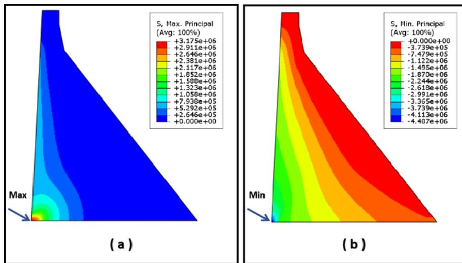
Figure 17 (a) Plot Contour of Highest Primary Stress at time 6.99 s, and (b) Plot Contour of Smallest Primary Stress at time 6.72 s (in Pa).
