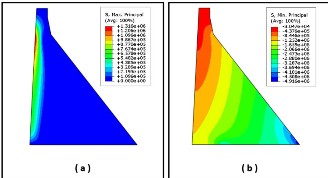
Figure 21 (a) Contour Plot of the Highest Principal Stress at 6.95 s, and (b) Contour Plot of the Lowest Principal Stress at 7.03 s (both in Pa).
