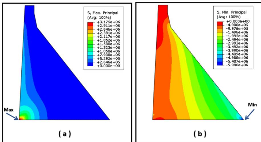
Figure 18 (a) Plot Contour of Highest Primary Stress at time 6.99 s, and (b) Plot Contour of Smallest Primary Stress at time 6.99 s (in Pa).
