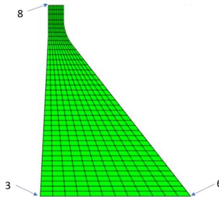
Figure 10 Nodal Point Coordinates at the Dam's Toe (6), Heel (3), and Crest (8).
