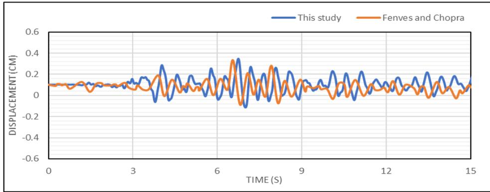
Figure 16 Toe Vertical Displacement (Nodal Point 6)
