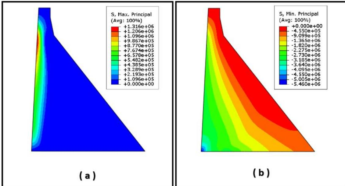
Figure 20 (a) Contour Plot of the Highest Principal Stress at 6.95 s, and (b) Contour Plot of the Lowest Principal Stress at 5.85 s (both in Pa).
