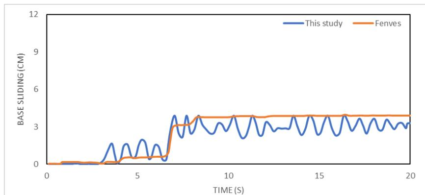
Figure 19 Abaqus Model Response with Base Sliding.
