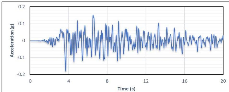
Figure 7 Unscaled Horizontal Component of the Taft Earthquake.
