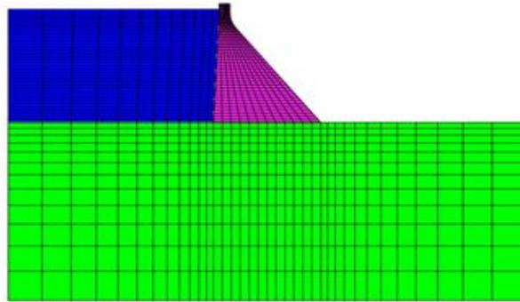
Figure 2 Abaqus Model Represents the System Consisting of the Dam, Foundation, and Reservoir.
