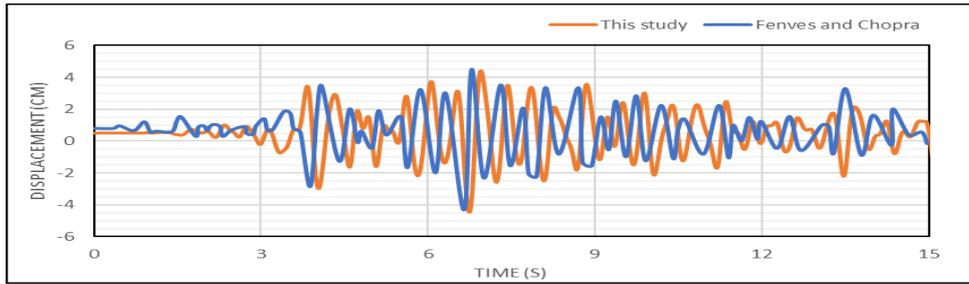
Figure 11 Crest Horizontal Displacement (Nodal Point 8)
