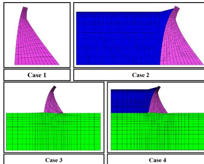
Figure 5 Mode Shapes of an Abaqus Model for Four Distinct Scenarios Utilizing Abaqus.
