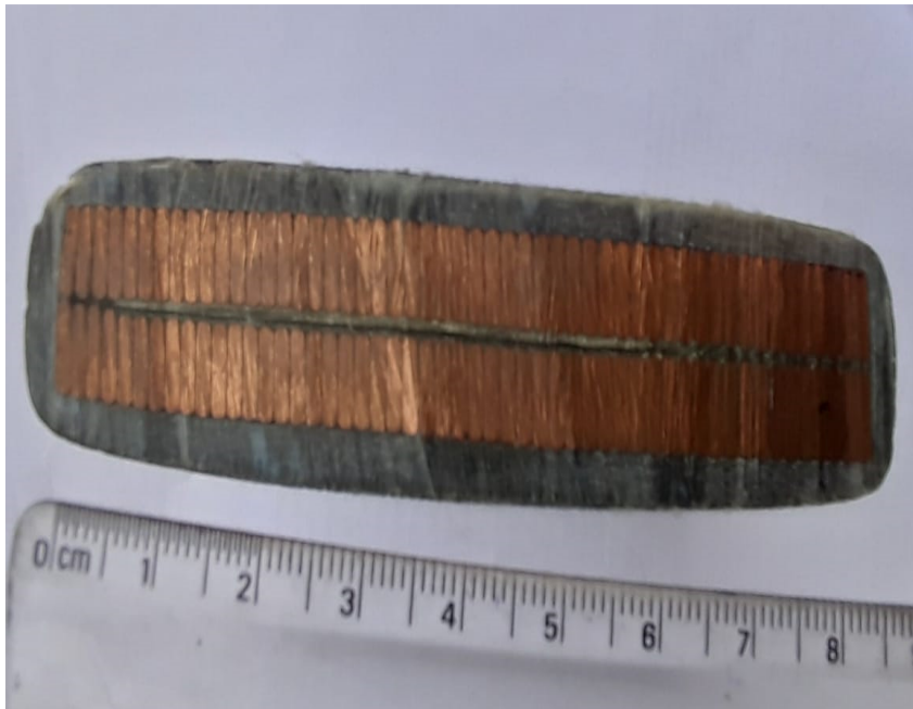
Fig. 5. Cross Section of the coil of a typical High Voltage 150 MW alternator winding.
