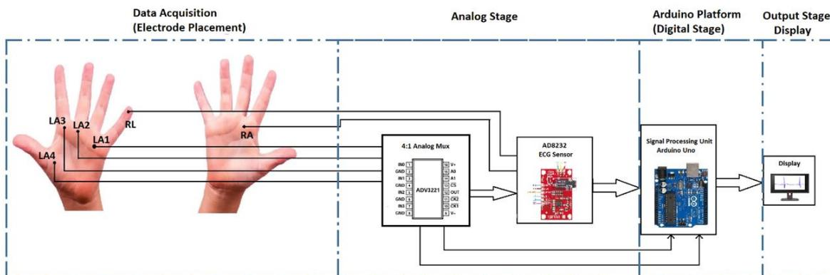
Figure 2. Electrode placement positioning and system Architecture
