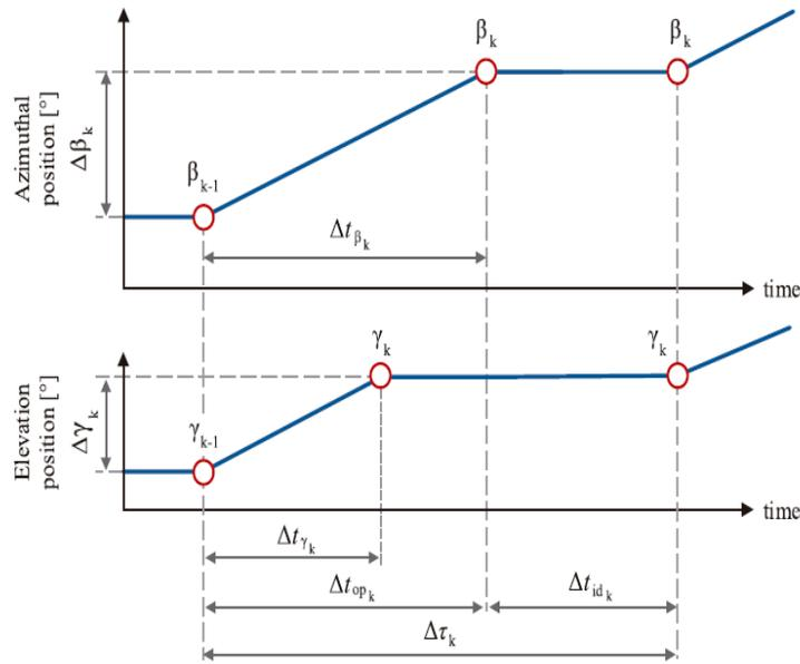
Figure 6: Time intervals for tracking movement from point
