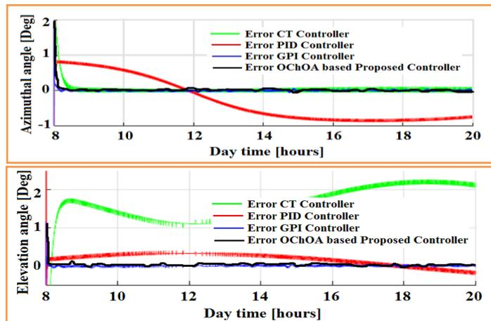
Figure 5: The trajectory's tracking accuracy
