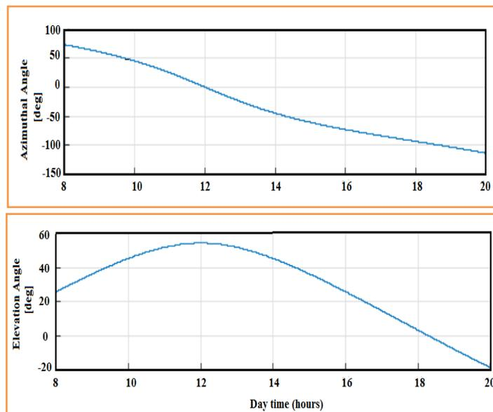
Figure 3: Solar path segmentation simulation for  $\epsilon_\beta=\epsilon_\gamma=0.25^\circ$ , and  $n_\beta=n_\gamma=788$ .
