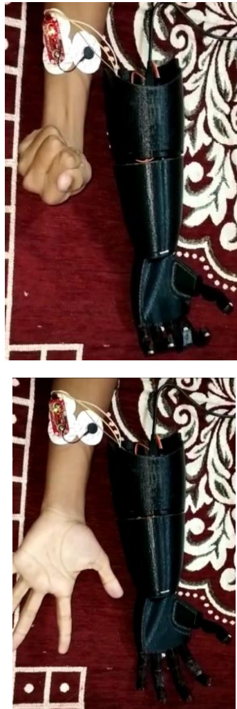
Figure. 8 Results of finger movement: (a) 3D printed hand (b) Hardware assembly on 3D printed hand (c) Closing of fingers (d) opening of fingers
