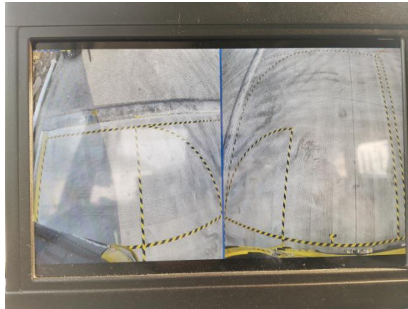
b) Field Verification Diagram of Class V and Class VI cameras Figure 8: Field Verification of Camera Field of View
