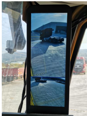
a) Field Verification Diagram of Class II and Class IV Cameras
