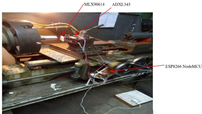
Fig. 2 - Placement of sensor on the lathe machine
