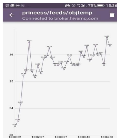
Fig. 9 - Output of Temperature as viewed on Smart Phone as graph
