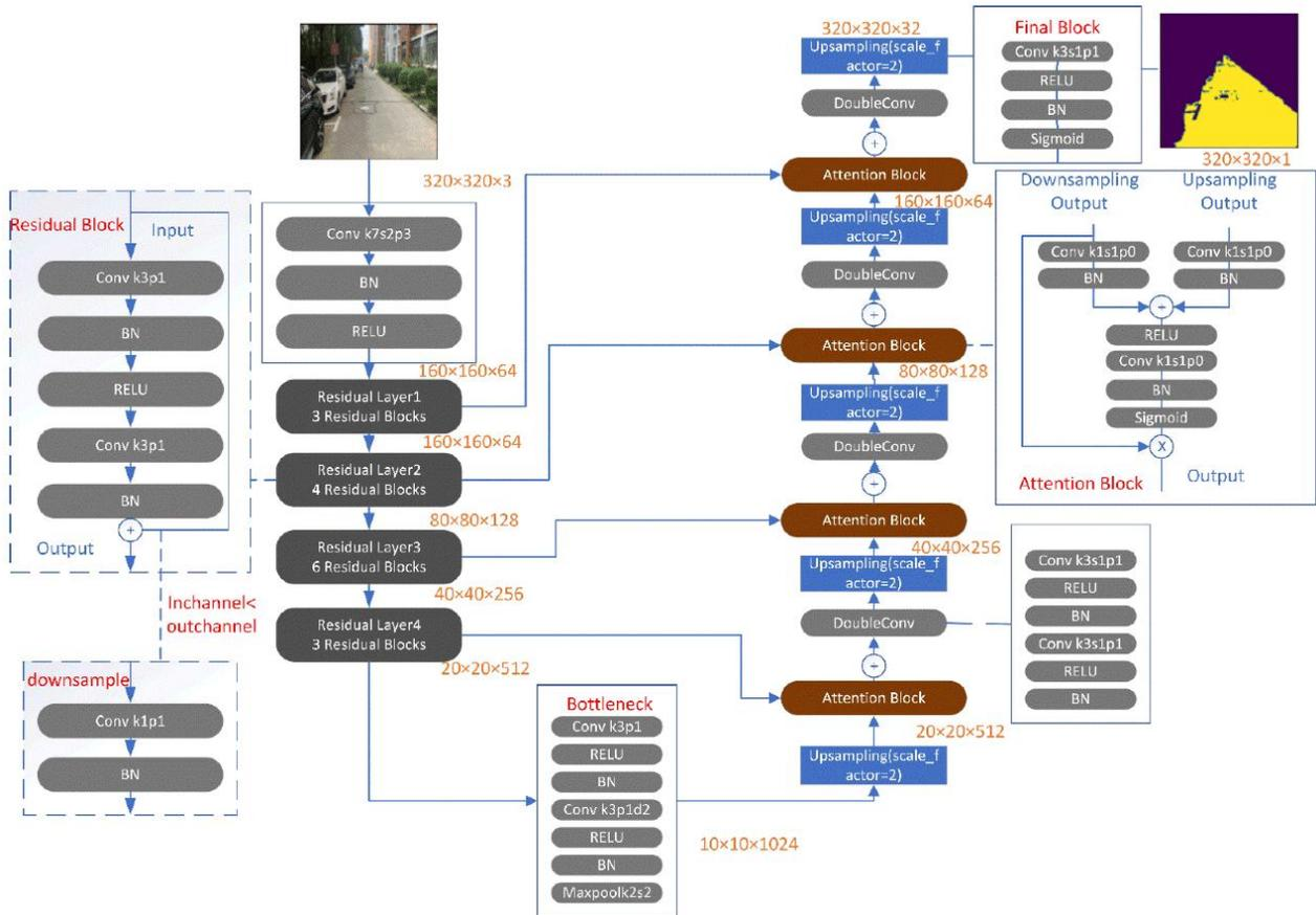
Fig.1 Schematic diagram of U-net model architecture
