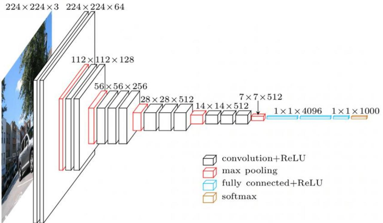
Fig. 2 VGG16 network structure diagram
