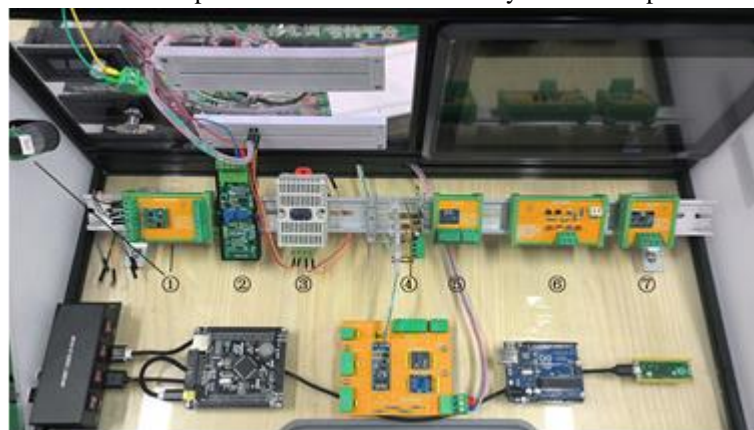
Figure 5: Physical diagram of the transducer access module layer
