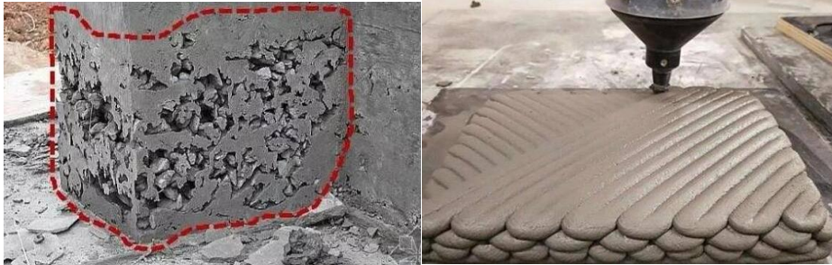
Figure 1: Typical Forms of Extrusion Breakage and Different Failure Patterns
