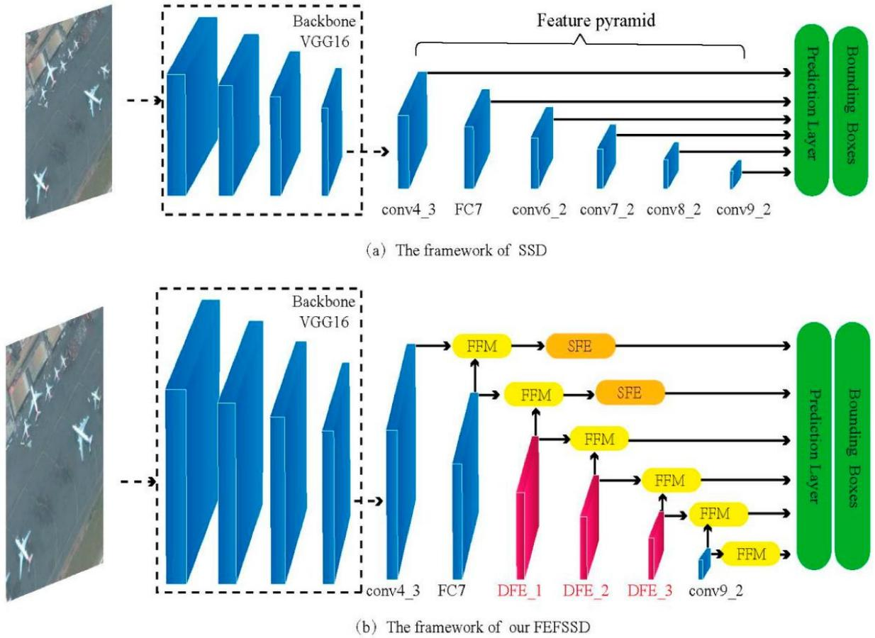
Fig.10 SSD algorithm structure diagram
