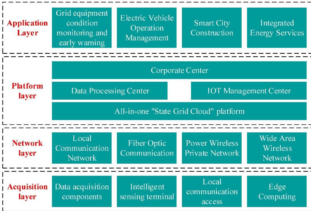
Fig.1 Transmission line monitoring system architecture
