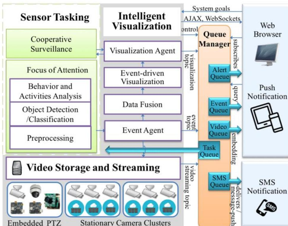
Fig.4 Interactive block diagram of the front-end modules of intelligent video surveillance
