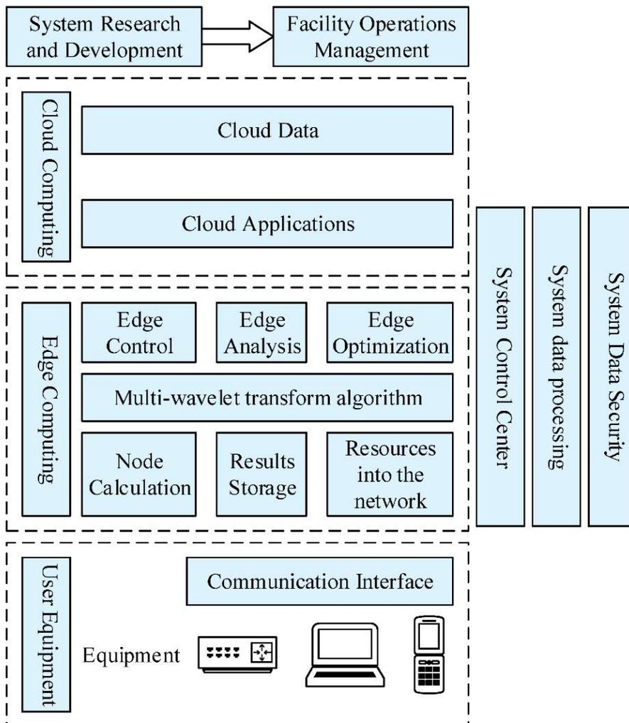
Fig.2 Hardware architecture of video monitoring extension machine
