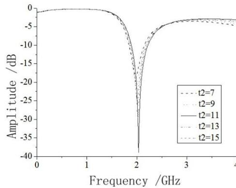
**Fig. 10.** The Changing curve of S parameter with adjusting the value of  $t_2$ --Changing curve of  $S_{22}$
