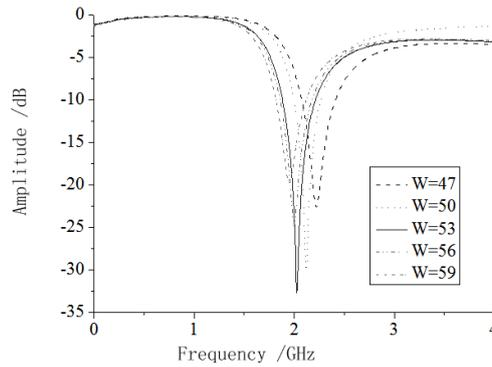
**Fig. 3.** The Changing curve of S parameter with adjusting the value of  $w$ --Changing curve of  $S_{11}$
