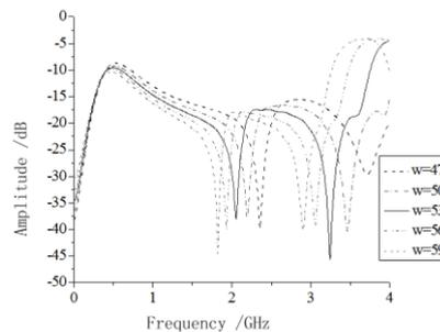
**Fig. 5.** The Changing curve of S parameter with adjusting the value of  $w$ --Changing curve of  $S_{21}$
