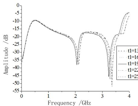
**Fig. 8.** The Changing curve of S parameter with adjusting the value of t1-- Changing curve of S21
