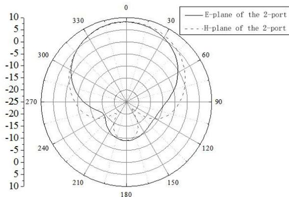
**Fig. 14.**The Simulation results of direction diagram after the optimization--Patterns of E-plane and H-plane of the 2-port
