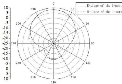
**Fig. 13.** The Simulation results of direction diagram after the optimization--Patterns of E-plane and H-plane of the 1-port
