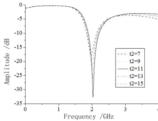
**Fig. 9.** The Changing curve of S parameter with adjusting the value of  $t_2$ --Changing curve of  $S_{11}$
