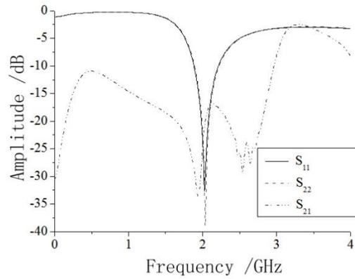
**Fig. 12.**Simulation values of S parameter after the optimization
