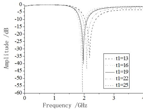
**Fig. 7.** The Changing curve of S parameter with adjusting the value of t1-- Changing curve of S22
