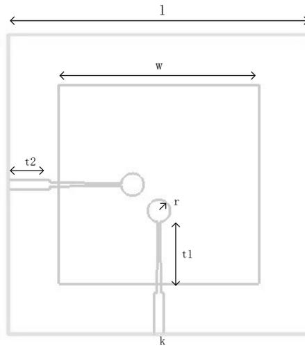
**Fig. 1.** Diagram of the unit structure --Structure diagram of double-polarized multilayer micro-strip antenna
