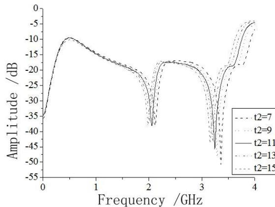
**Fig. 11.** The Changing curve of S parameter with adjusting the value of  $t_2$ --Changing curve of  $S_{21}$
