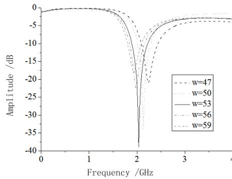
**Fig. 4.** The Changing curve of S parameter with adjusting the value of  $w$ --Changing curve of  $S_{22}$
