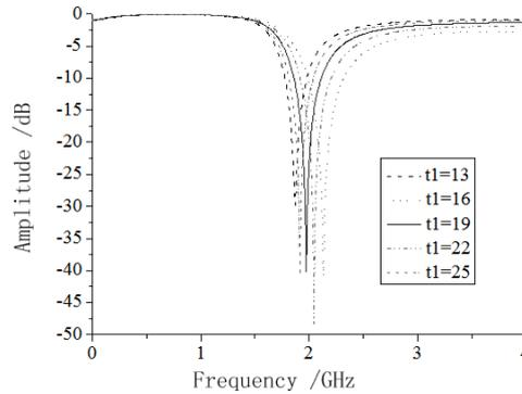
**Fig. 6.** The Changing curve of S parameter with adjusting the value of t1-- Changing curve of S11
