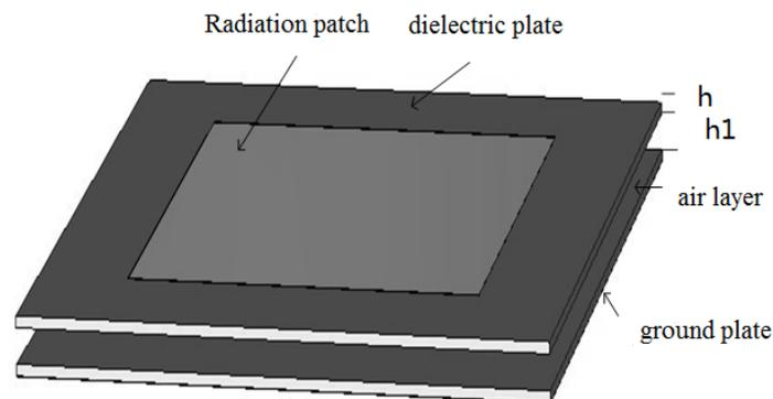
**Fig. 2.** Stereogram of the unit--Structure diagram of double-polarized multilayer micro-strip antenna
