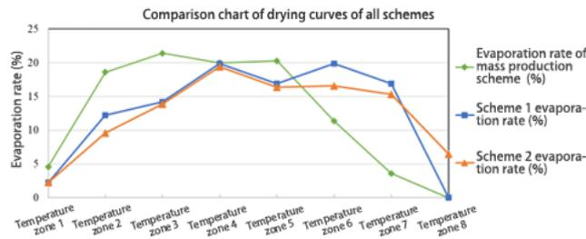
Figure 6: Comparison Chart of Drying Curves of All Schemes
