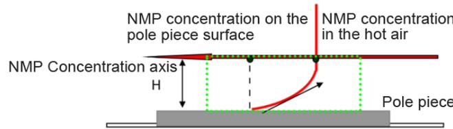
Figure 2: Schematic Diagram of the Evaporation Process of Nmp (Moisture) From the Surface of the Electrode to Hot Air
