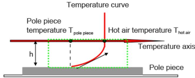
Figure 1: Schematic Diagram of Heat Transfer in the Drying Process of Pole Piece
