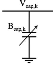
Fig.1 Connection of capacitor at bus-k for compensation
