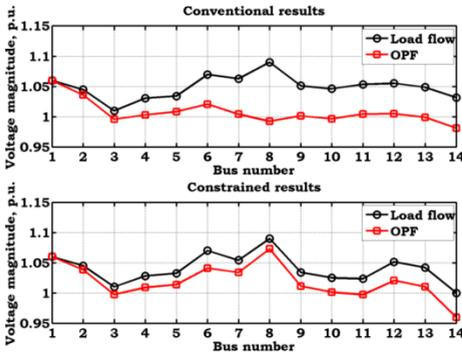
Fig.8 Variation of voltage magnitudes with OPF in conventional and constrained results of IEEE-14 bus system
