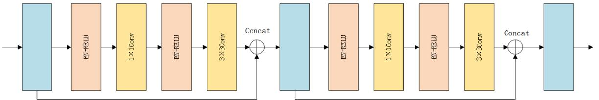
Figure 3: Architecture of DenseNet-100
