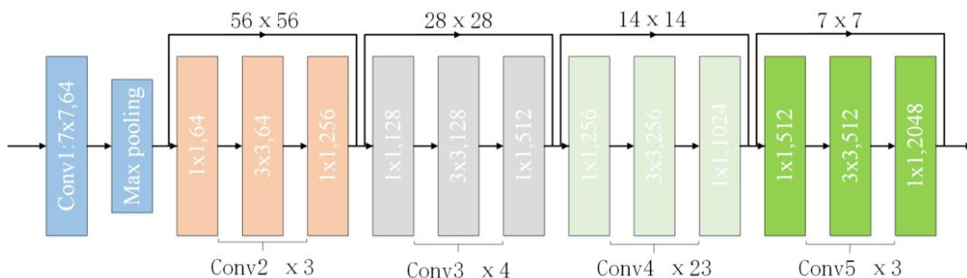
Figure 2: Structure Diagram of ResNet-101 Network
