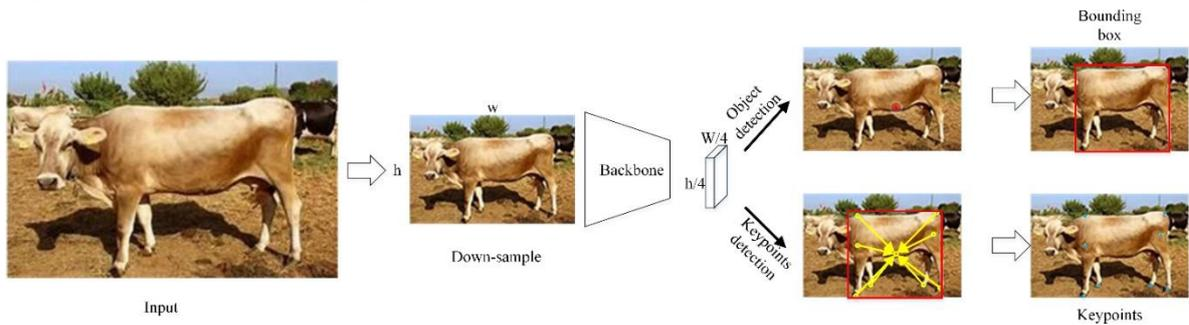
Figure 1: Block Diagram of CenterNet
