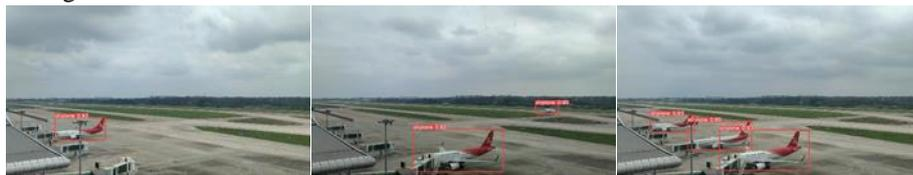
Figure 14: Detection Performance of YOLOv5-Aircraft with Different Aircraft Numbers
