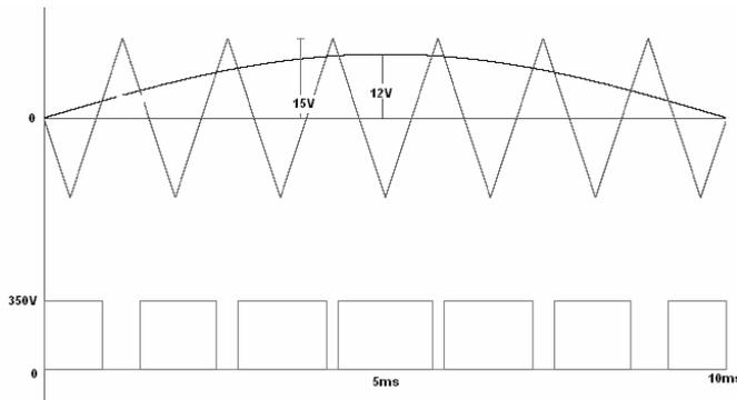
Figure 6. PWM fundamental and carrier waveforms (top) and produced pulse train (bottom) for  $m_{PWM}=0.8$ .
