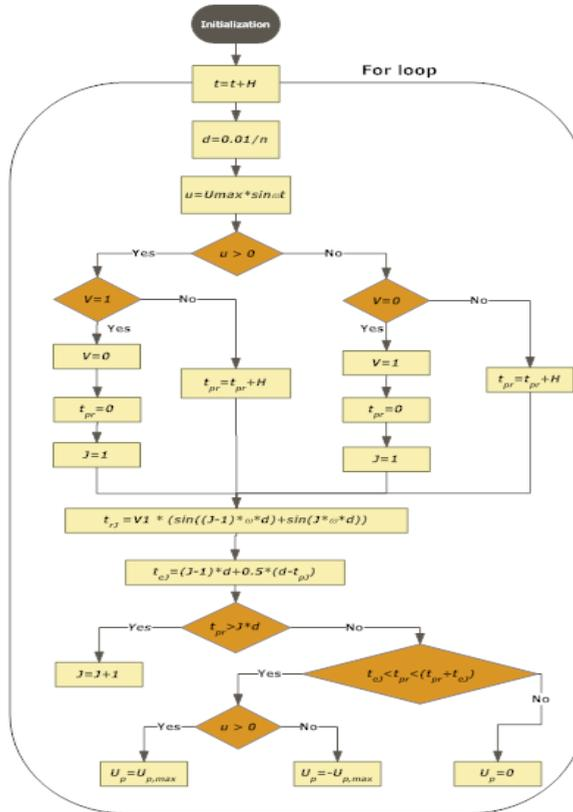
Figure 2. Flowchart for the calculation of pulses' duration and firing times for the proposed PWM strategy.
