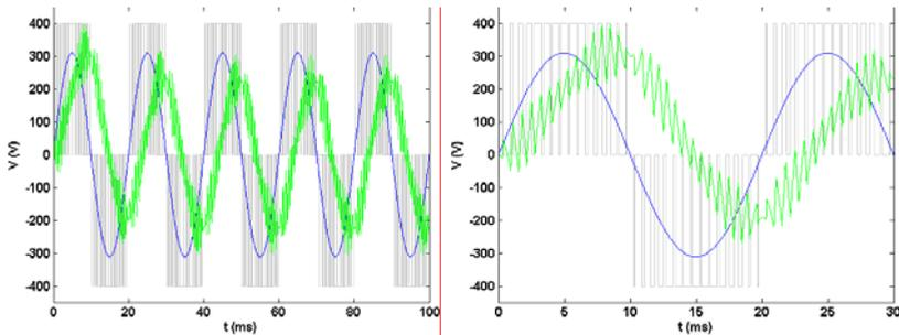
Figure 12. Simulation results for  $n=15$ . Right plot zooms in interval 0-30ms of left plot. Grey lines represent PWM pulse sequence.
