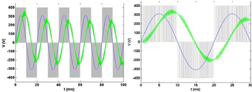
Figure 11. Simulation results for  $n=45$ . Network waveform (blue line), produced waveform (green line) and PWM pulse sequence (grey lines). Right plot zooms in interval 0-30ms of left plot.
