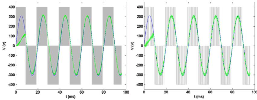
Figure 13. (a) Simulation results for  $n=45$  (left) and (b) for  $n=15$  (right) with  $\varphi=22^\circ$  and  $L=0.04H$ . Voltage (black line) and produced waveform (green line) are in phase. Grey areas represent dense PWM pulse sequence
