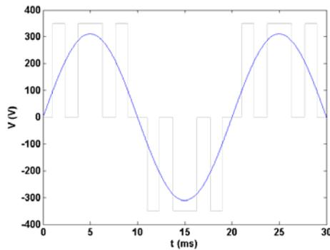
Figure 3. Simulation of network voltage waveform (blue line) by PWM sequence (grey line) for  $n=3$ .
