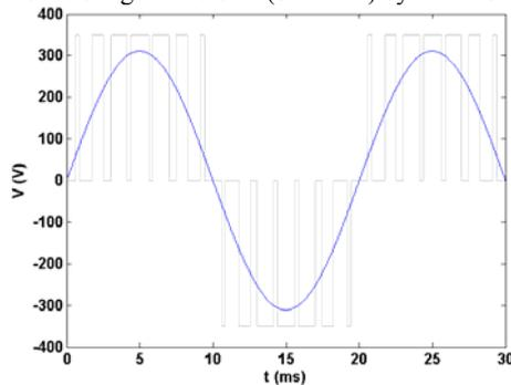
Figure 4. Simulation of network voltage waveform (blue line) by PWM sequence (grey line) for  $n=7$ .
