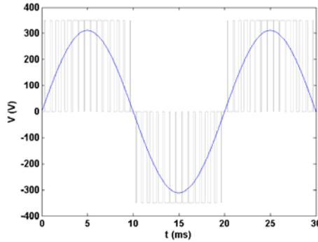
Figure 5. Simulation of network voltage waveform (blue) by PWM sequence (grey line) for  $n=15$ .
