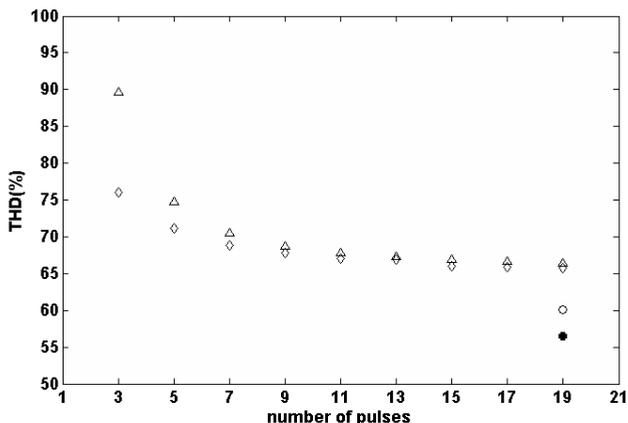
Figure 7. THD vs. number of pulses per period for different modulation indexes.  $m_{PWM}=0.8$  (diamonds),  $m_{NPWM}=0.8889$  (triangles),  $m_{PWM}=0.89333$  (open circle) and  $m_{NPWM}=0.972$  (solid circle).
