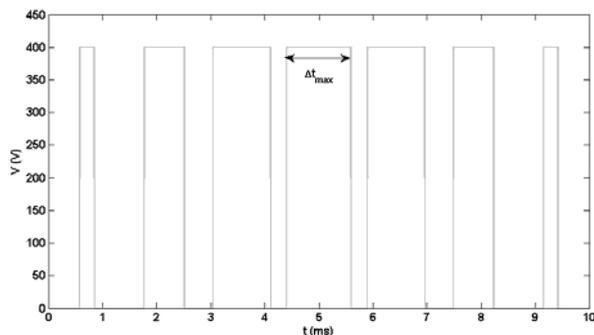
Figure 8. Definition of the maximum pulse width ( $\Delta t_{max}$ ) for a pulse train (gray solid line) with odd number (here  $n=7$ ) of pulses.
