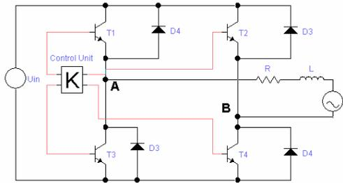
Figure 9. Block diagram of the circuit used to deliver power (from P/V systems) to network. This circuit used for the simulation.
