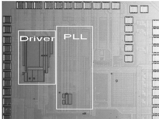
Figure.6 The die micrograph of the transmitter
