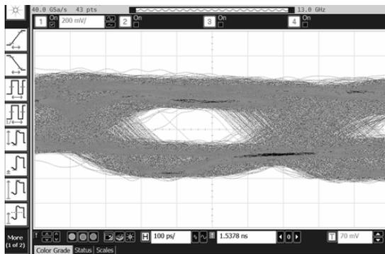
Figure.8 The eye diagram of the LVDS with conventional pre-emphasis at 1.5Gb/s(Horizontal axis = 100ps/div, vertical axis=100mV/div)
