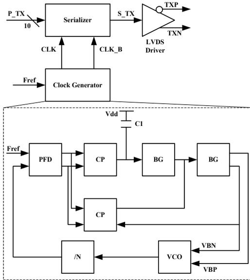
Figure. 1 Transmitter system block diagram
