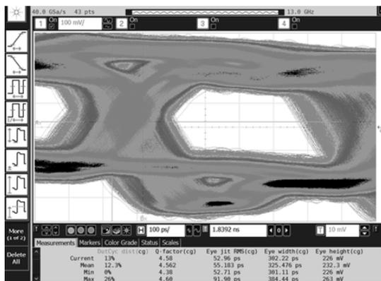
Figure.9 The eye diagram of the LVDS with improved pre-emphasis at 1.5Gb/s (Horizontal axis = 100ps/div, vertical axis=100mV/div) .
