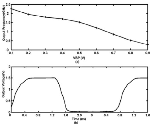
Figure.3 (a) The tuning sensitivity of VCO (b) The transient simulation waveform of the VCO
