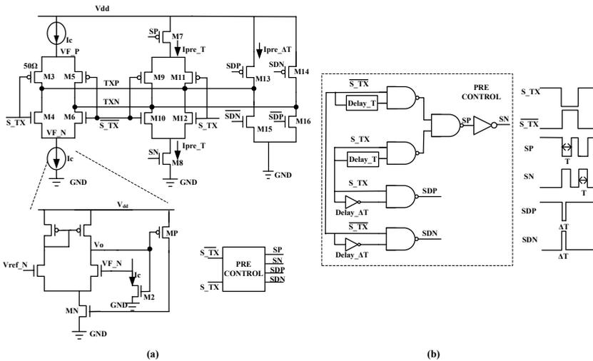
Figure.4 The circuit schematic of the LVDS driver (a) The schematic of the LVDS driver (b) Pre-emphasis control circuit and its signal waveform
