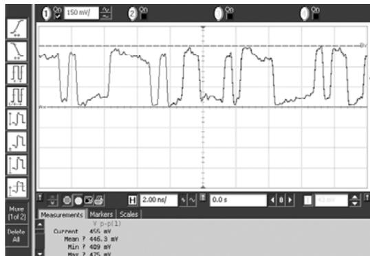
Figure.7 The waveform of the LVDS with improved pre-emphasis at 1.5Gb/s
