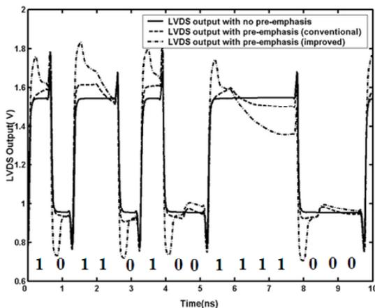
Figure.5 The simulation results of the LVDS output
