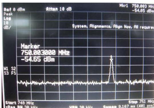
Figure.10 The spectrum of the recovery clock
