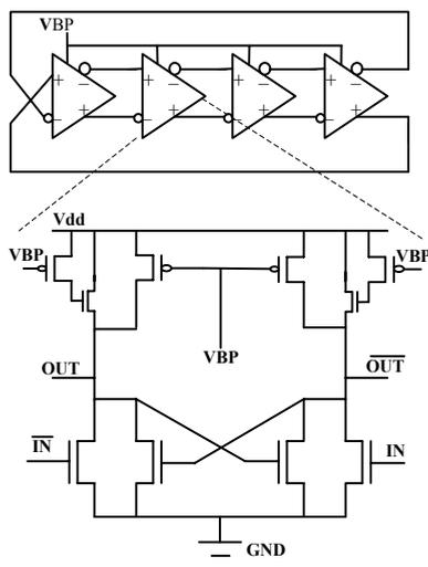
Figure. 2 The circuit schematic of VCO
