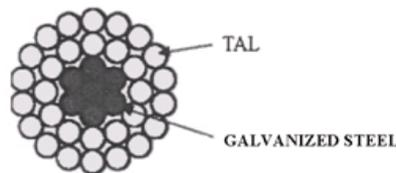
Fig. 1. Cross section's TACSR conductor.
