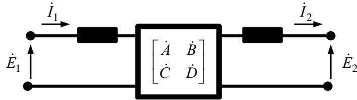
Fig. 6. Line equivalent quadrupole.
