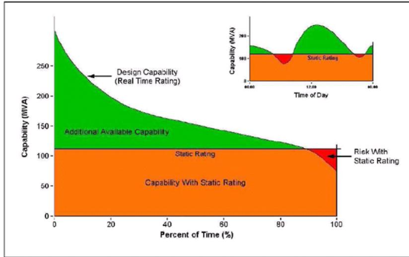
Fig. 5. Static and dynamic rating capability.
