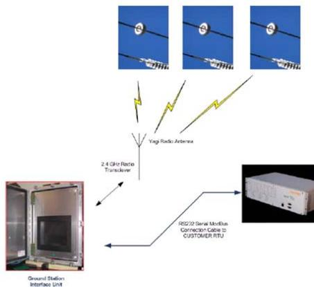
Fig. 14. Radio transmission system 2,4 GHz standard “ZigBee”.
