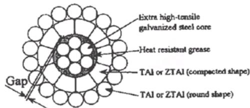
Fig. 2. Cross section's Gap-type conductor.
