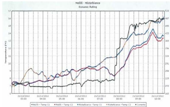
Fig. 21. Load current and temperature conductor trends.
