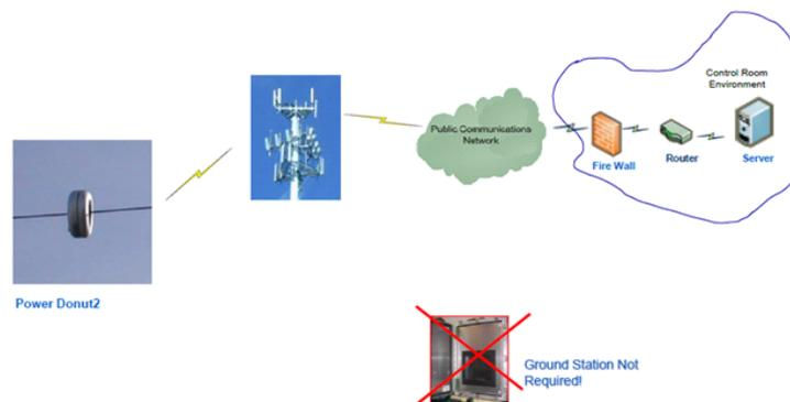
Fig. 13. Data transmission system through GSM/GPRS/EDGE.
