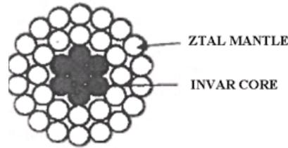
Fig. 3. Cross section's ZTACIR conductor.
