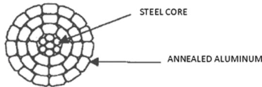
Fig. 4. Cross section's ACSS/TW conductor.
