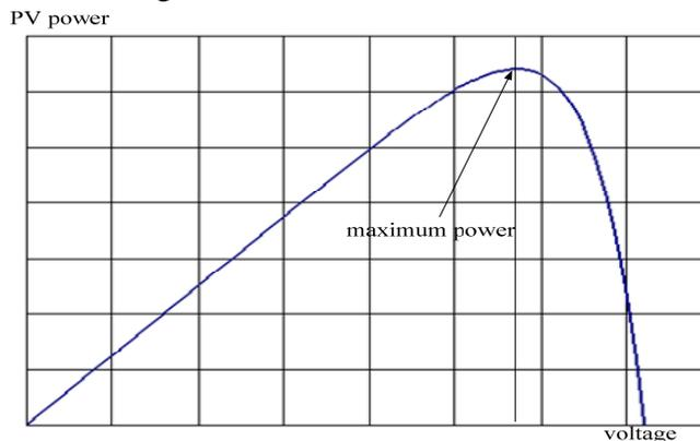
Fig. 1. Characteristic of PV array.
