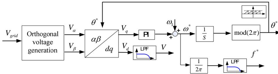
Figure 2. General structure of a single-phase grid-connected inverter PLL
