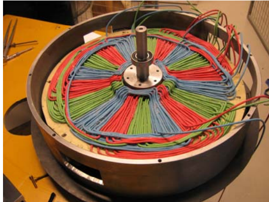
Figure 12. View of the stator of the three phase axial flux prototype.
