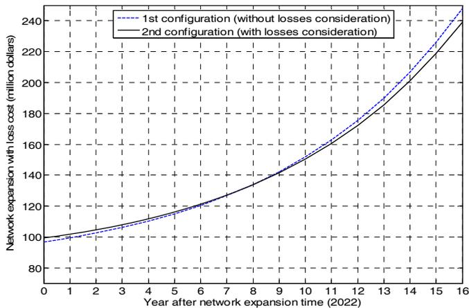
Figure 9. Sum of expansion costs and annual losses cost of the network with the two proposed configurations
