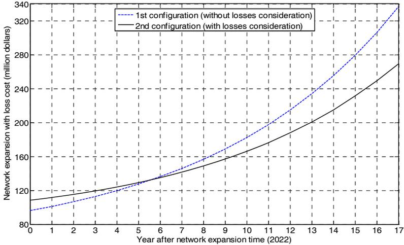
Figure. 6. : Sum of expansion costs and annual losses cost of the network with the two proposed configurations in scenario 2
