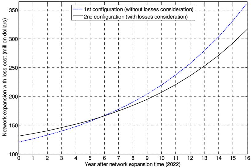
Figure. 4. : Sum of expansion costs and annual losses cost of the network with the two proposed configurations in scenario 1
