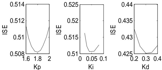
Figure 5. Performance index ISE of gas turbine plant
