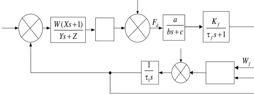
Figure 1. Transfer function model of gas turbine plant.
