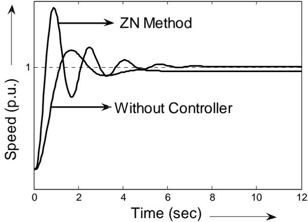
Figure 4. Response of gas turbine plant without controller and with PID controller tuning using ZN method – A Comparison.
