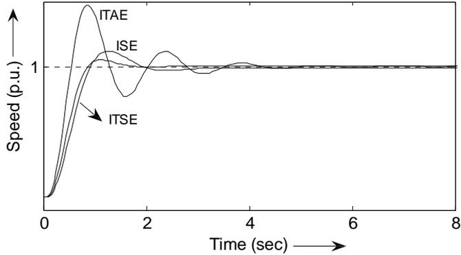
Figure 8. Comparison of gas turbine plant response with PID controller, tuned using ISE, ITAE and ITSE.
