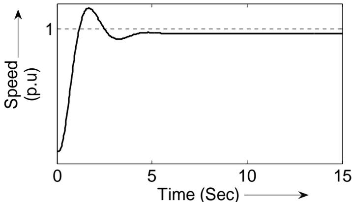
Figure 3. Response of gas turbine plant without secondary controller
