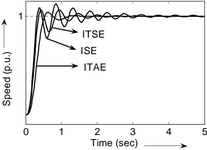
Figure 9. Comparison of gas turbine plant response with various PID controllers tuned using various fitness functions in GA.
