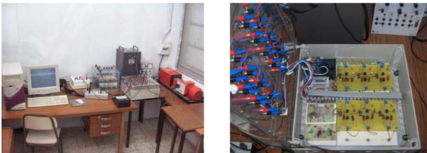
Fig. 12: General view of the platform and the electronic cards module.
