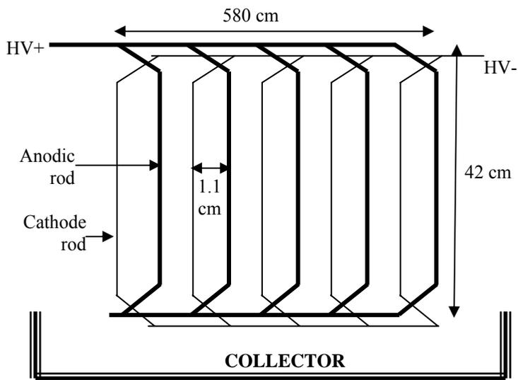
Figure 2: Descriptive diagram of the "electric netting"
