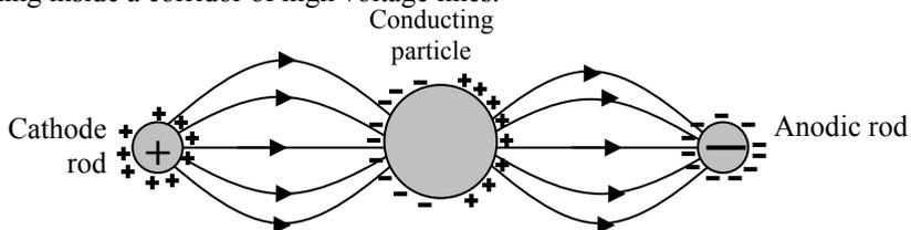
Figure 6: Charges induced on a conducting particle
