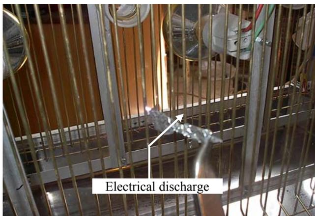
Figure 5: Simulation of the electric discharge using an aluminium end
