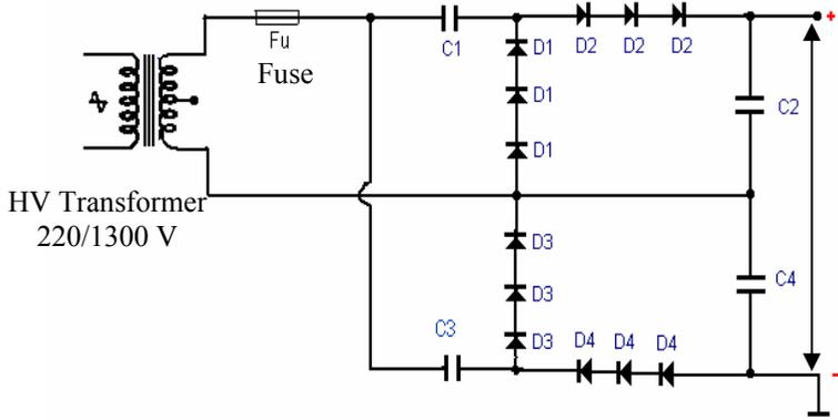
Figure 3: Electrical circuit of the high voltage supply
