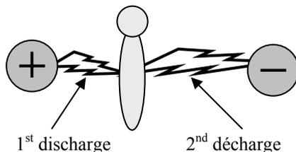
Figure 7: Electrical discharge occurring between the insect and electrodes
