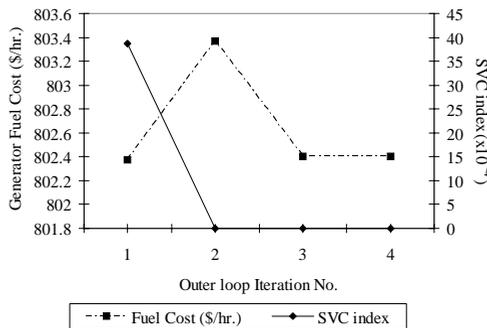
Figure 3: Outer loop convergence characteristic of SADE\_ALM for case 1.
