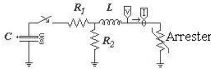
Figure 1. Typical measuring setup for ZnO surge arresters.
