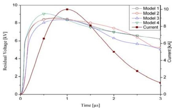
Figure 9. Response to 10kA, 1/2μs for the surge arresters of reference [4].
