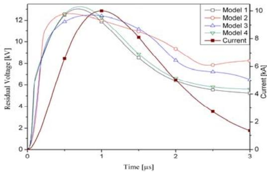
Figure 12. Response to 10kA, 1/2μs for the surge arresters of reference [18]
