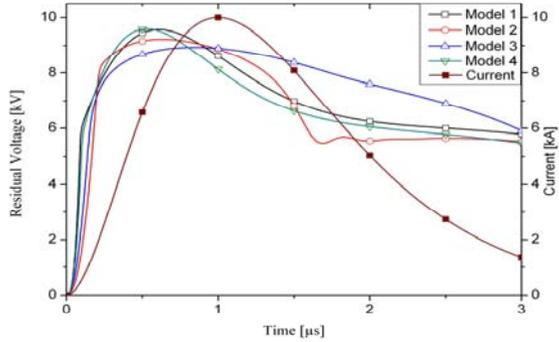
Figure 11. Response to 10kA, 1/2μs for the surge arresters of reference [17]
