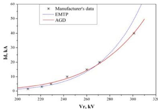
Figure 3. Comparison with the EMTP and the data of the manufacturers for surge arresters 108kV.
