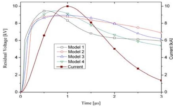
Figure 10. Response to 10kA, 1/2μs for the surge arresters of reference [5].
