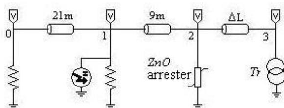
Figure 13. Typical protection scheme by surge arresters.
