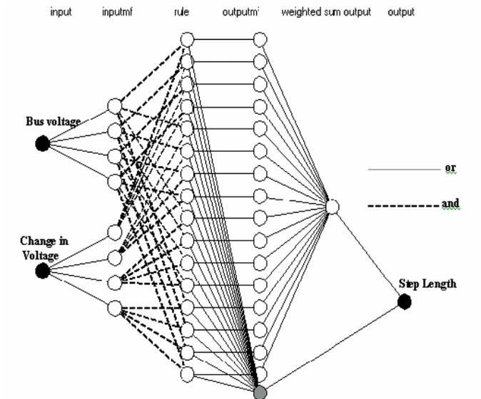
Figure 3. Architecture of ANFIS Step Length Controller
