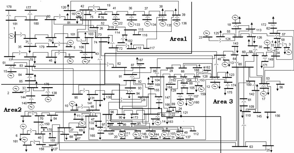
Figure 7. Single line diagram of Indian 181 bus system
