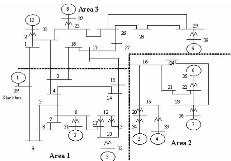
Figure 6. Single line diagram of New England 39 bus system
