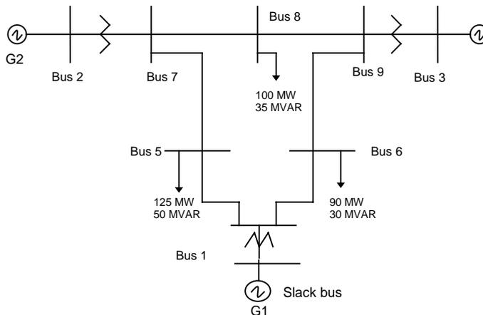
Figure 5. Single line diagram of WSCC 9 bus system
