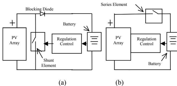
Fig.1 Regulator designs: (a) Shunt Controller, (b) Series Controller
