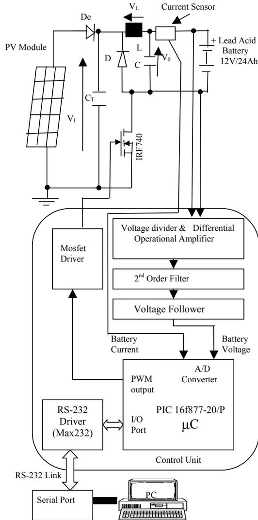
Fig. 6: Detailed diagram of the proposed system.
