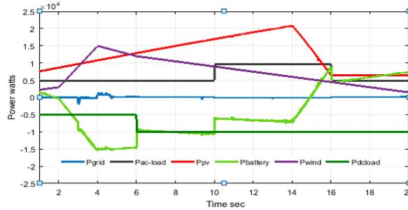
Fig.8. Power flows in MG for 20<SOC<90
