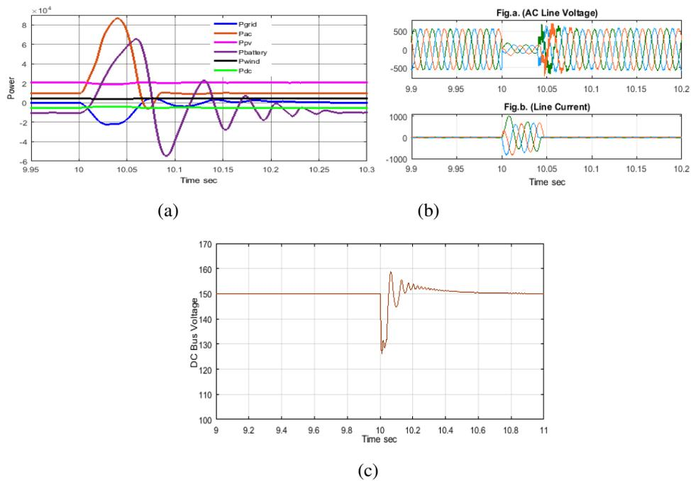
Fig.12. a) Power flows in the MG, b) 400V AC bus voltage and fault current, c) DC bus voltage
