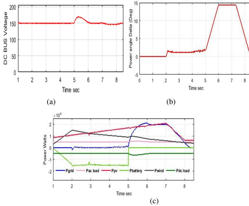
Fig.13. a) DC bus voltage, b) Power angle delta profile, c) Power flows in the MG
