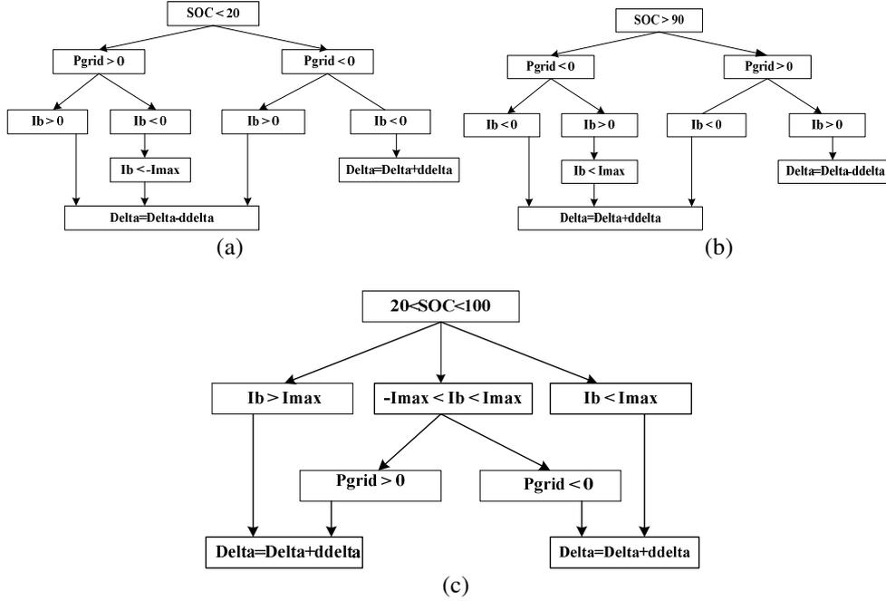
Fig.7. Power flows Algorithms for the MG system a) SOC < 20, b) SOC > 90, c) 20 < SOC < 90
