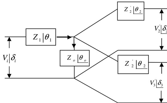
Fig.4. Equivalent circuit
