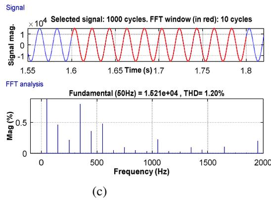
Fig.14. : (a) Phase voltage and line voltage of TBMLI, ( b) THD of 400 AC Voltage without filter (c) THD of 11kV AC voltage with filter.
