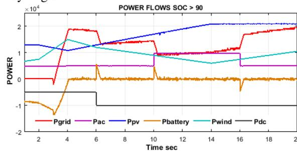
Fig.9. Power flows in MG for SOC > 90
