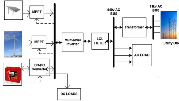
Fig.1. General Architecture of microgrid
