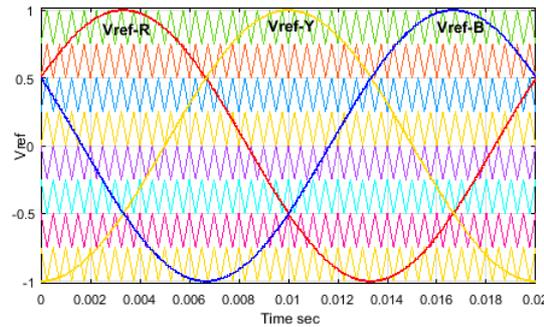
Fig.5. Multi-carrier PWM technique
