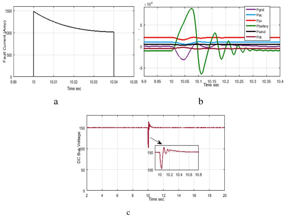
Fig.11. a) DC Fault current, b) Power oscillations in MG, c) DC bus voltage
