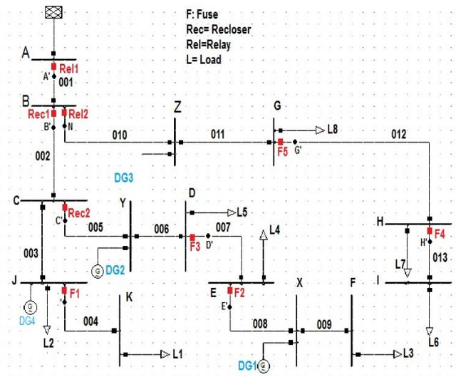
**Fig 6. Single line diagram of the typical test network.**
