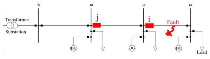
**Fig 4. Different DG unit installation in a radial grid**
