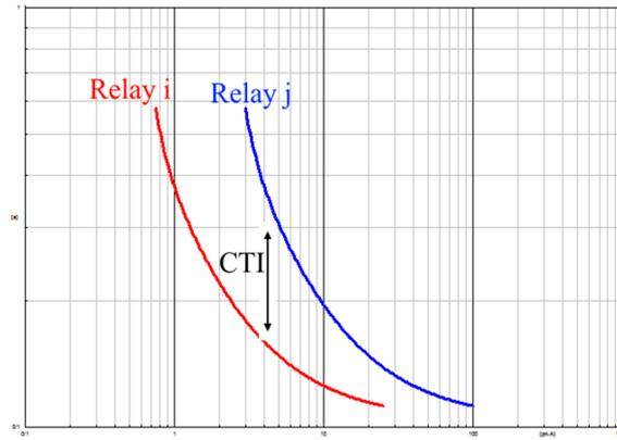
**Fig 5. Relay-relay coordination**
