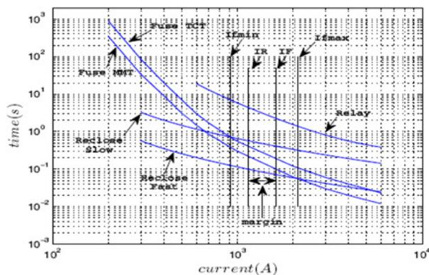
**Fig 3. Recloser-fuse-relay CA**
