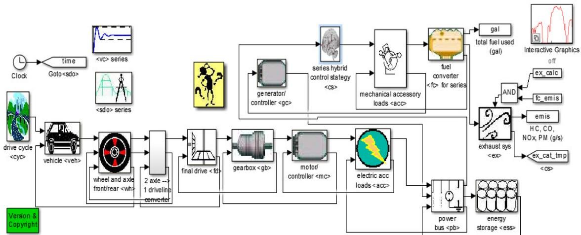
Fig. 3. Block diagram of SHEV
