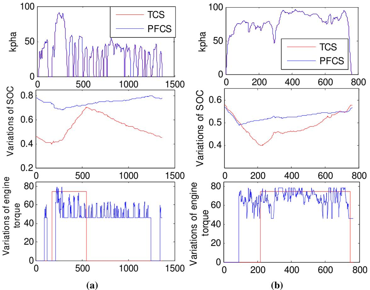
Fig. 8. Battery SOC history and engine torque in the (a) UDDS and the (b) HWFET driving cycles
