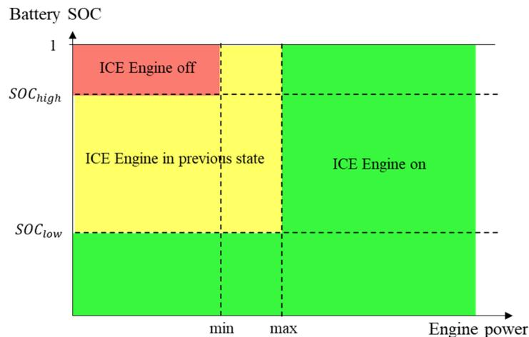
Fig. 5. Battery state of charge in PFCS
