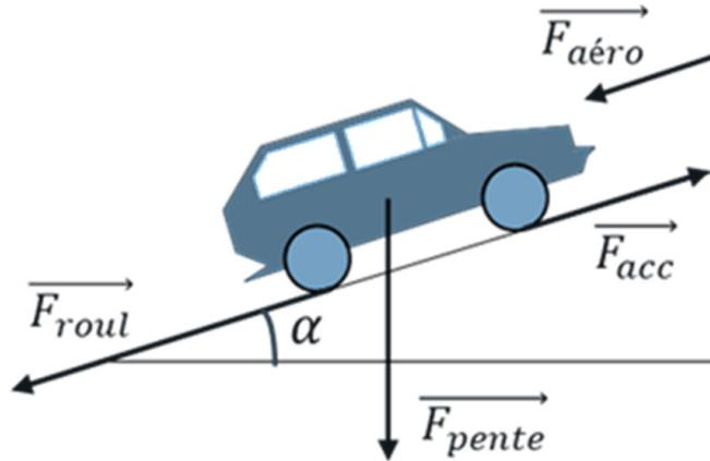
Fig. 2. Forces acting to the vehicle
