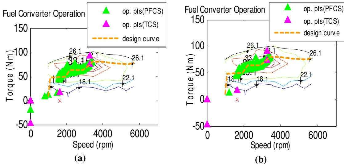
Fig. 9. Engine operating points in the (a) UDDS and the (b) HWFET driving cycles
