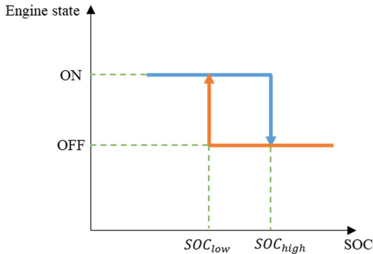
Fig. 4. Engine state in TCS
