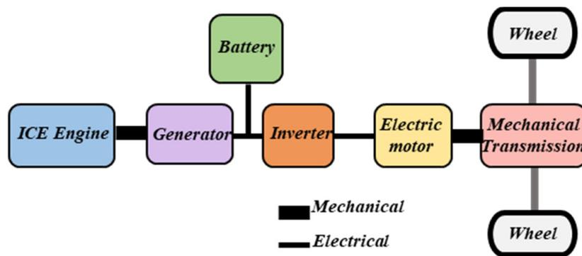
Fig. 1. Configuration of the SHEV
