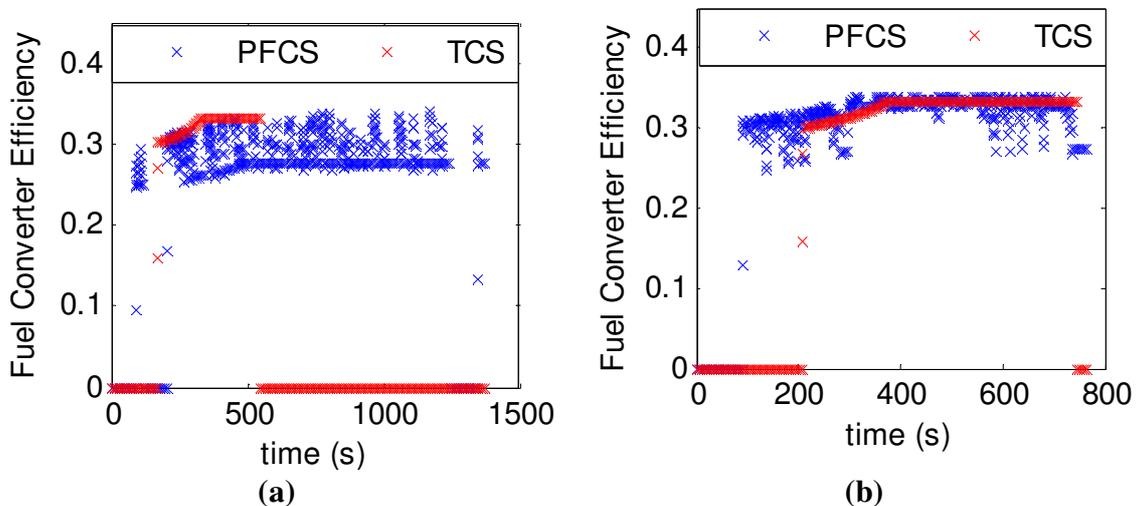
Fig. 10. Fuel converter efficiency in the (a) UDDS and (b) HWFET driving cycles
