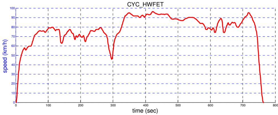
Fig. 7. HWFET cycle speed profile
