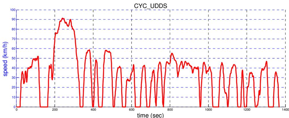
Fig. 6. UDDS cycle speed profile
