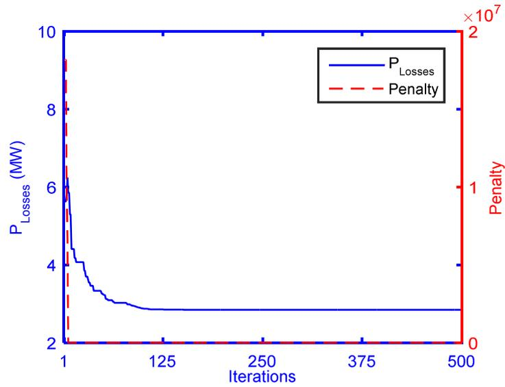
Figure 4 : Active power losses minimization.
