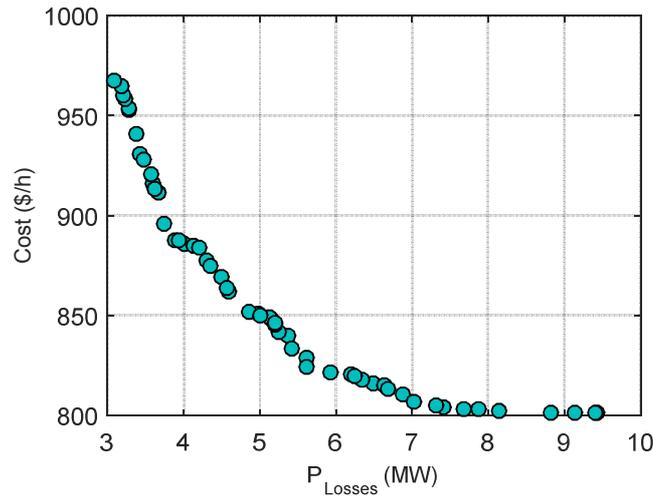
Figure 8 : Pareto optimal set of solutions for CASE-8.
