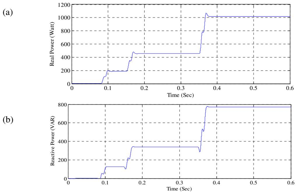
**Fig. 7.** (a) Real power to loads and (b) reactive power to loads from the inverter
