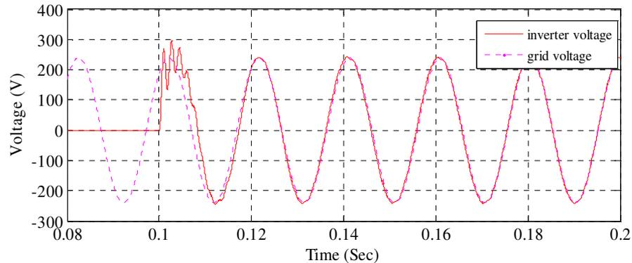
**Fig. 19.** The inverter is connected with microgrid of 240V at 51Hz at 0.1s and it is synchronized in nearly 0.18s using PLL
