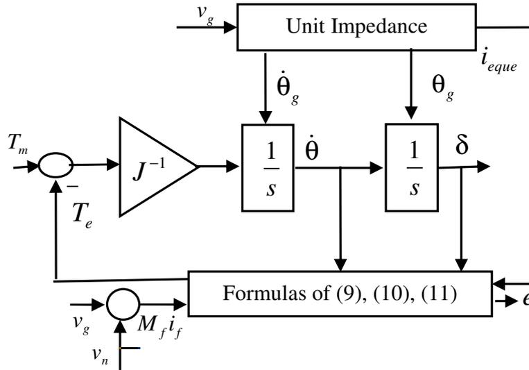
**Fig. 5.** The VSCon controller connecting microgrid voltage and frequency
