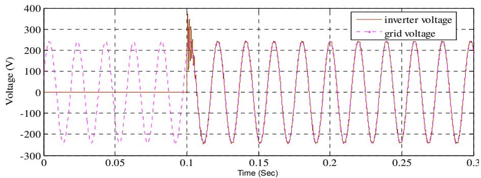
**Fig. 12.** The inverter and grid voltage are synchronized at 0.1s when voltage phase is shifted by  $10^0$  at 51Hz.
