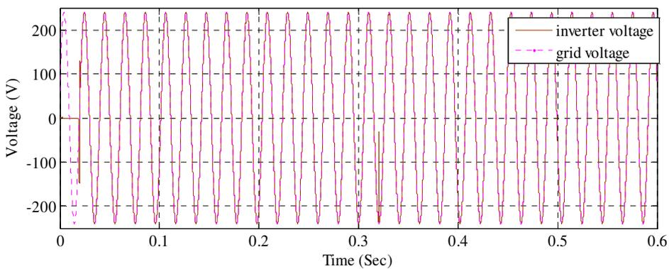
**Fig. 18.** Grid-inverter voltage while connecting non-linear load
