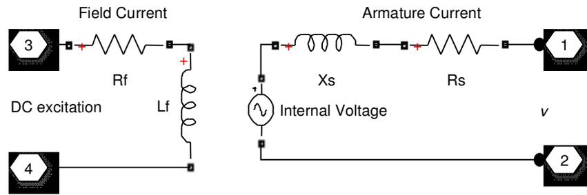
**Fig. 3.** Equivalent of Single-phase SG
