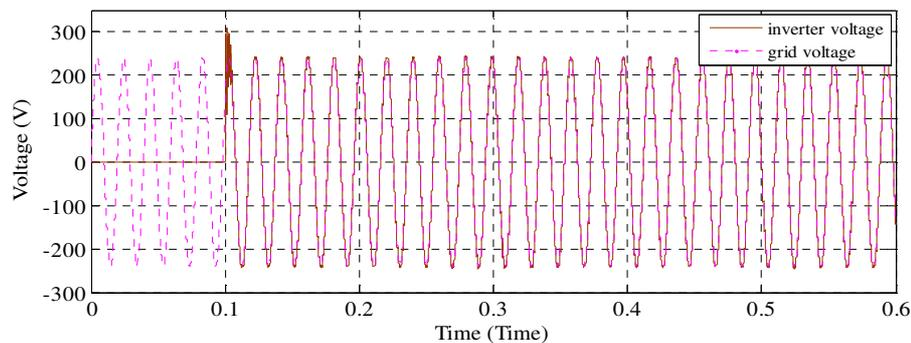
**Fig. 9.** The microgrid voltage and inverter voltage are synchronized at 0.1s
