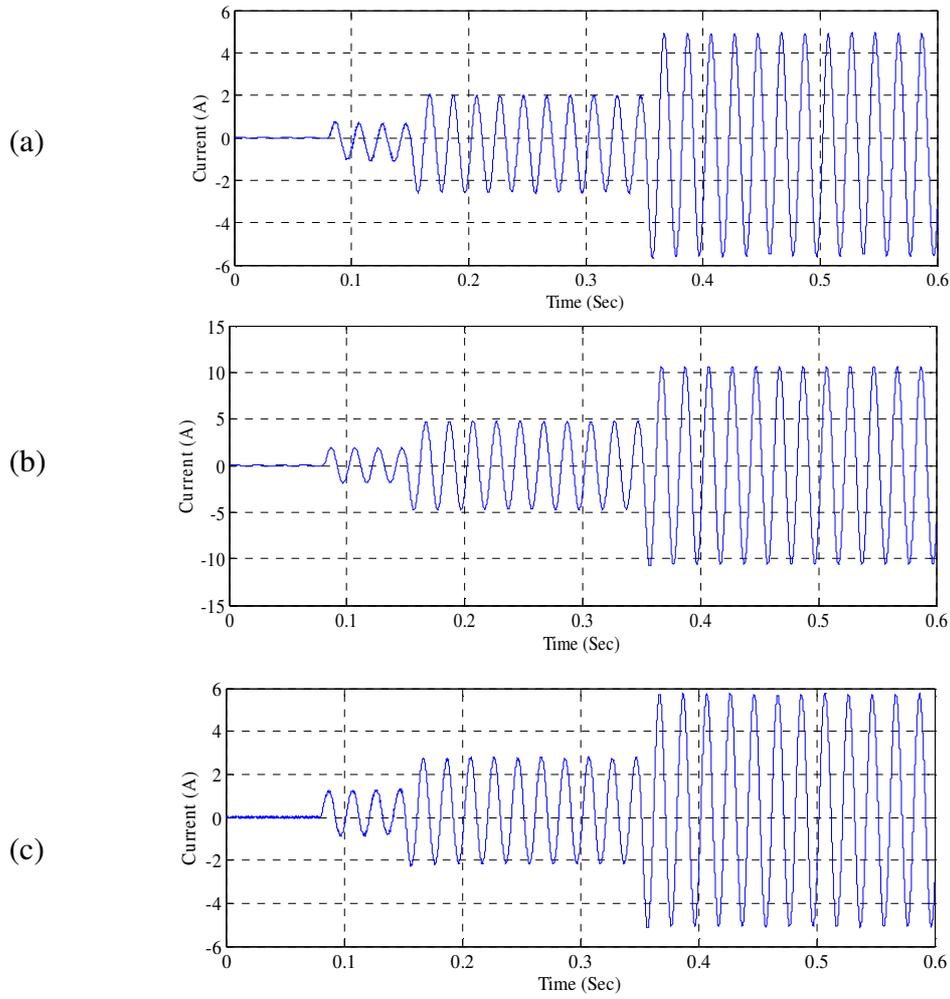
**Fig. 6.** (a) Current supply by the inverter to the loads, (b) grid current supplied to loads at PCC, (c) total current consumed by loads
