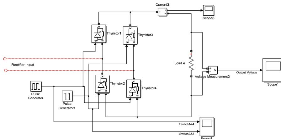
**Fig. 15.** Rectifier as a non-linear load.
