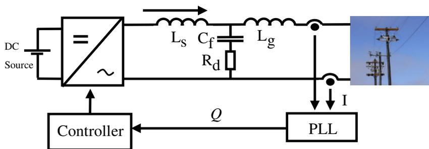
**Fig. 1.** PLL synchronization technique in low voltage-level microgrid- inverter.
