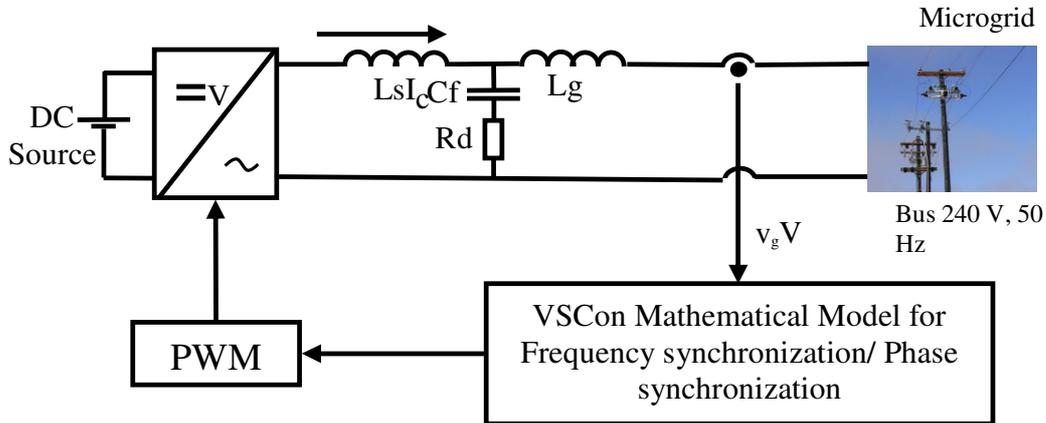
**Fig. 4.** Block diagram of VSCon without PLL structure.
