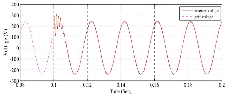
**Fig. 20.** The inverter is connected with microgrid of 240V at 51Hz at 0.1s and it is synchronized in nearly 0.12s using VSCon
