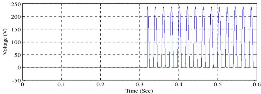
**Fig. 17.** Voltage drop across the non-linear load
