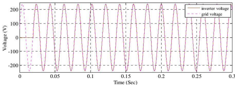
**Fig. 14.** Grid-inverter voltage respond when Load 1, Load 2 and Load 3 are been connected
