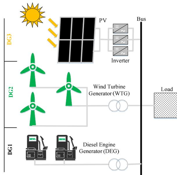
Figure 1. Simplified schematic of islanded microgrid
