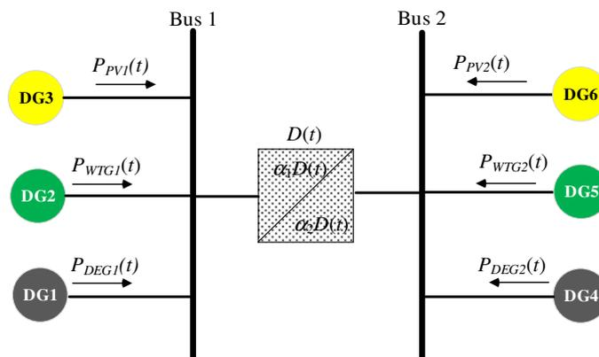
Figure 4. Power flow of islanded microgrid
