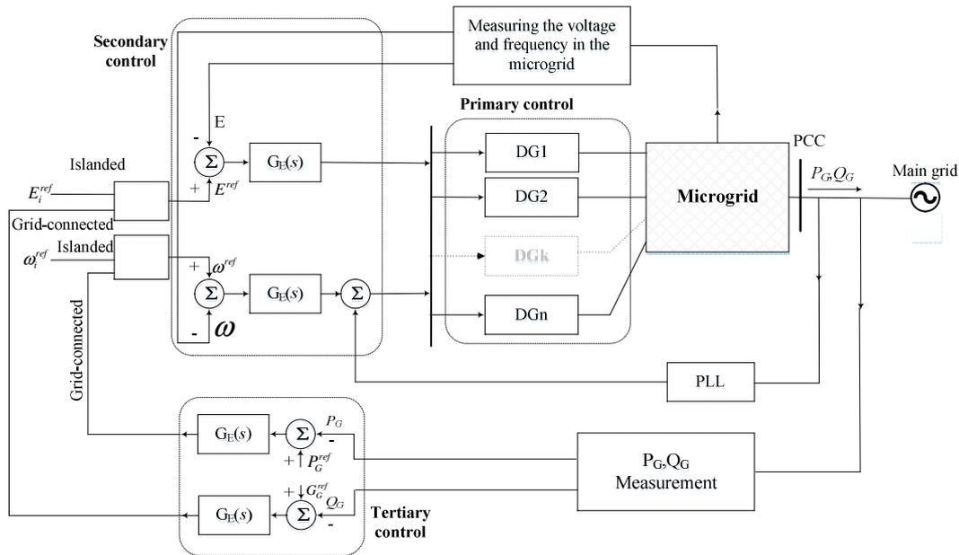
Figure 3. Block diagram of secondary and tertiary controls [6]
