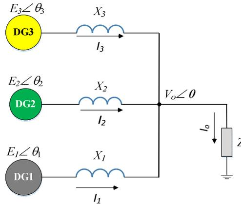
Figure 2. Equivalent circuit of three parallel-connected DGs
