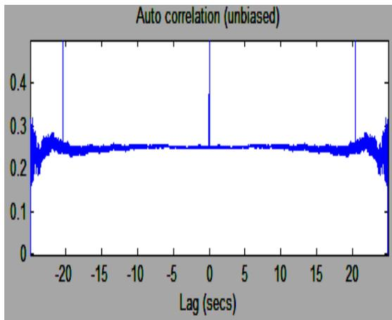
Figure 3: Autocorrelation function of the generated PN code.
