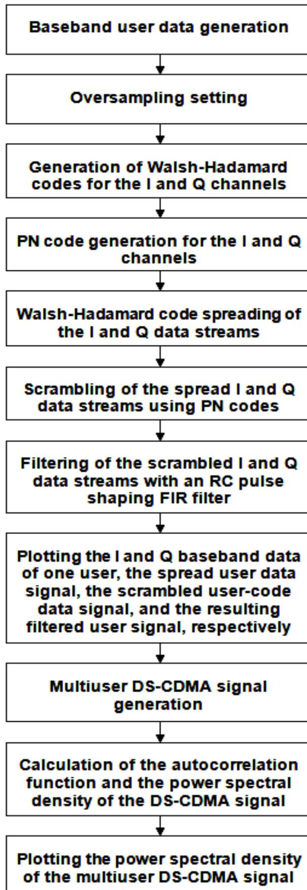
Figure 1: Flowchart of the simulation procedure of multiuser DS-CDMA signal generation in MATLAB.
