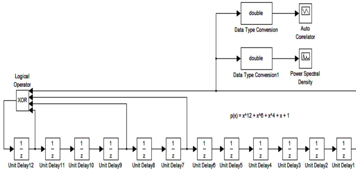
Figure 2: Proposed and simulated PN generator based on the 12-stage linear feedback shift register for PN code generation in MATLAB.
