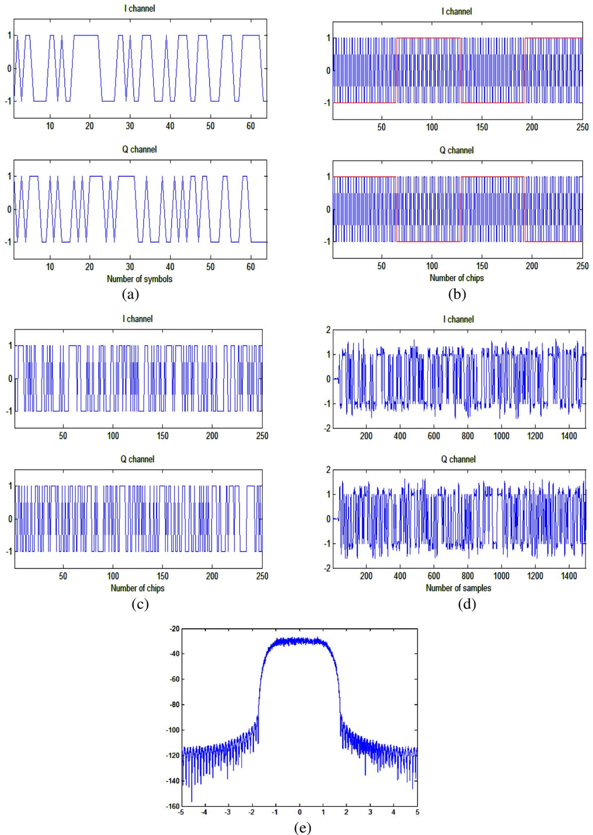
Figure 5: Simulation results of DS-CDMA signal generation. (a)  $I$  and  $Q$  baseband data of one user, (b) User data after spreading by Walsh-Hadamard code, (c) User-coded data after scrambling by a PN code, (d) Resulting filtered user signal by a baseband RC filter, and (e) Power spectral density of a multiuser DS-CDMA signal.
