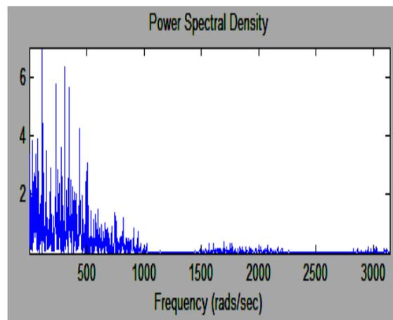
Figure 4: Power spectral density of the generated PN code.
