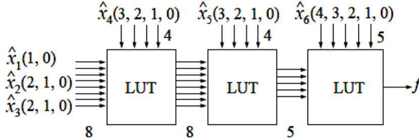
Figure 7: LUT cascade for error detection function.
