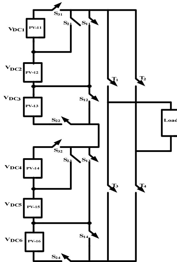
Fig. 1. Equivalent Structure of Single Phase PV system fed 13-level DCLMLHBI
