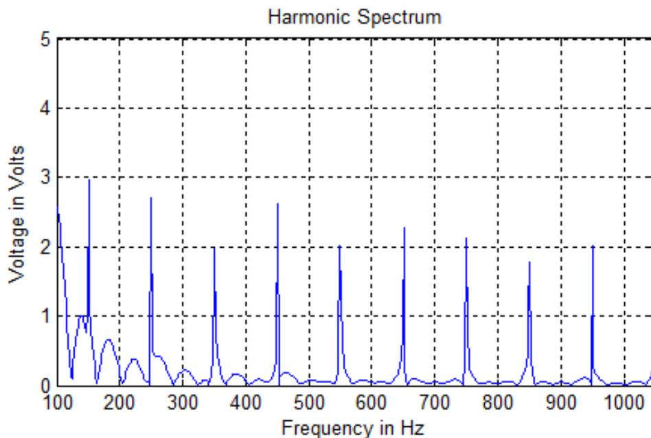
Fig. 5. Individual Order Voltage Harmonic Analysis (Single Phase)
