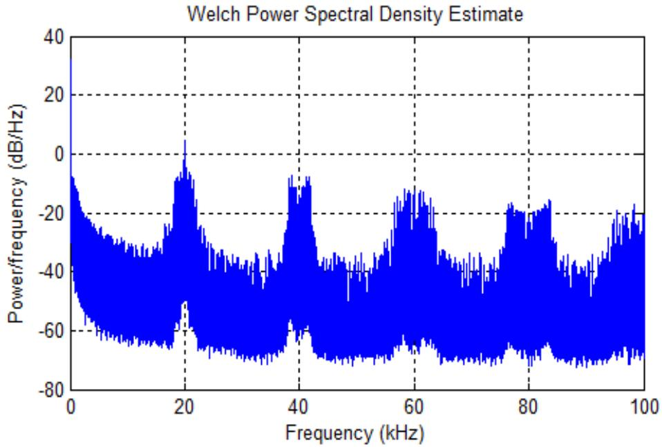
Fig. 6. Output Voltage Power Density Spectrum (Single Phase)
