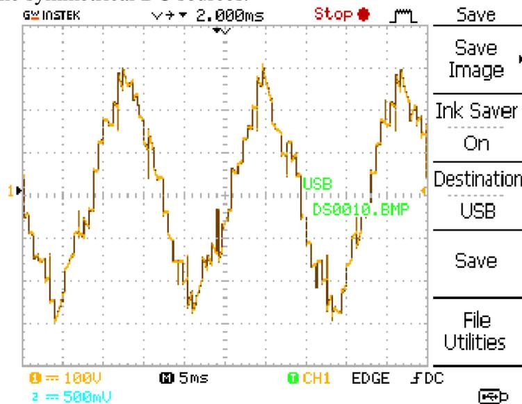
Fig. 9. Experimented Output Voltage of DCLMLHBI
