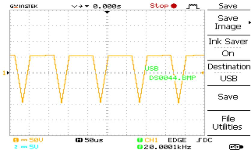
Fig. 7. SPWM Pulse to  $S_{11}$
