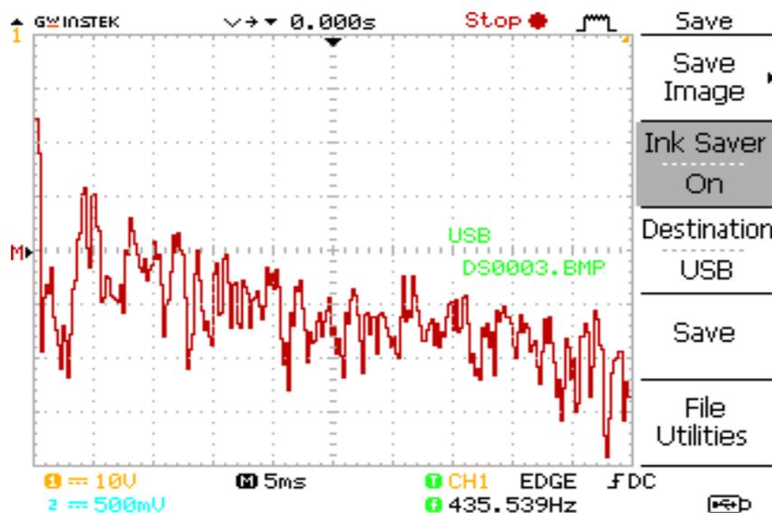
Fig. 10. Output voltage FFT analysis of single-phase DCLMLHBI
