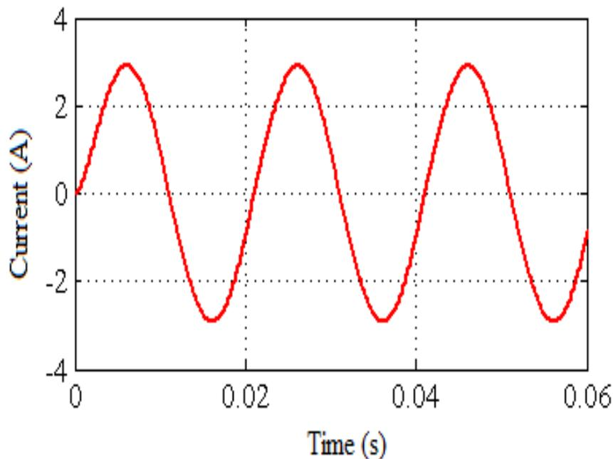
Fig. 3. Load Current (Single Phase)
