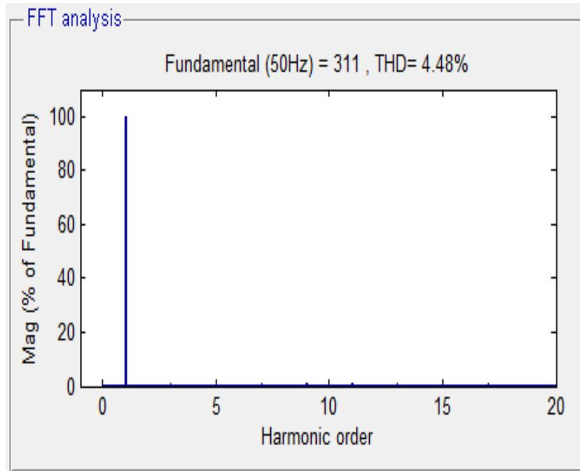
Fig. 4. Output Voltage THD Spectrum (Single Phase)
