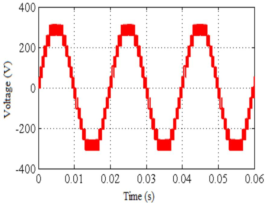
Fig. 2. Inverter Output Voltage of Single Phase DCLMLHBI System
