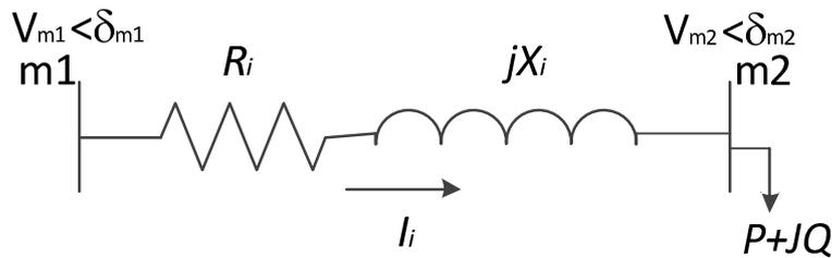
Figure 1. One-line diagram of the two-bus radial distribution system.
