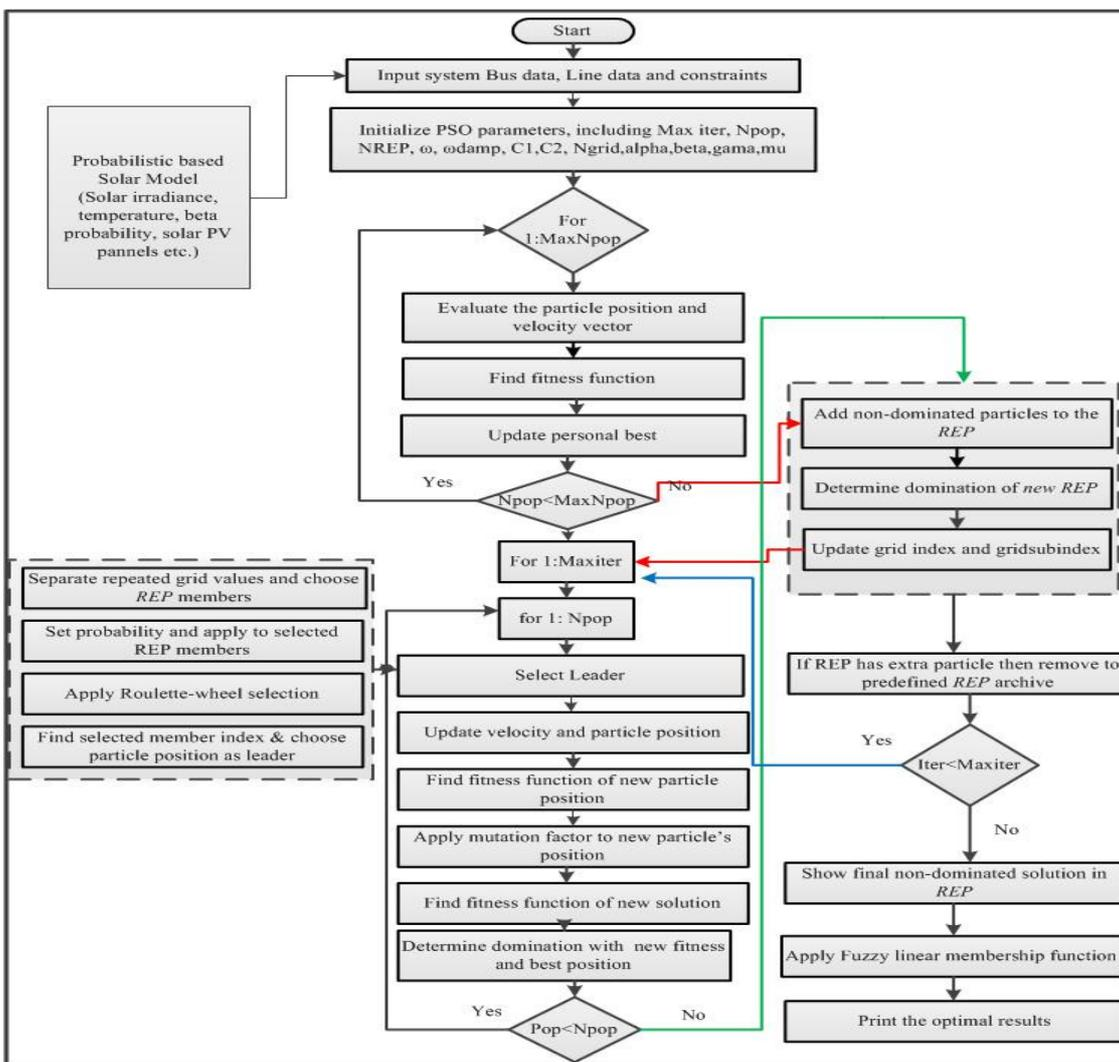
Figure 2. Flow chart for optimal placement of solar power DG using MOPSO.
