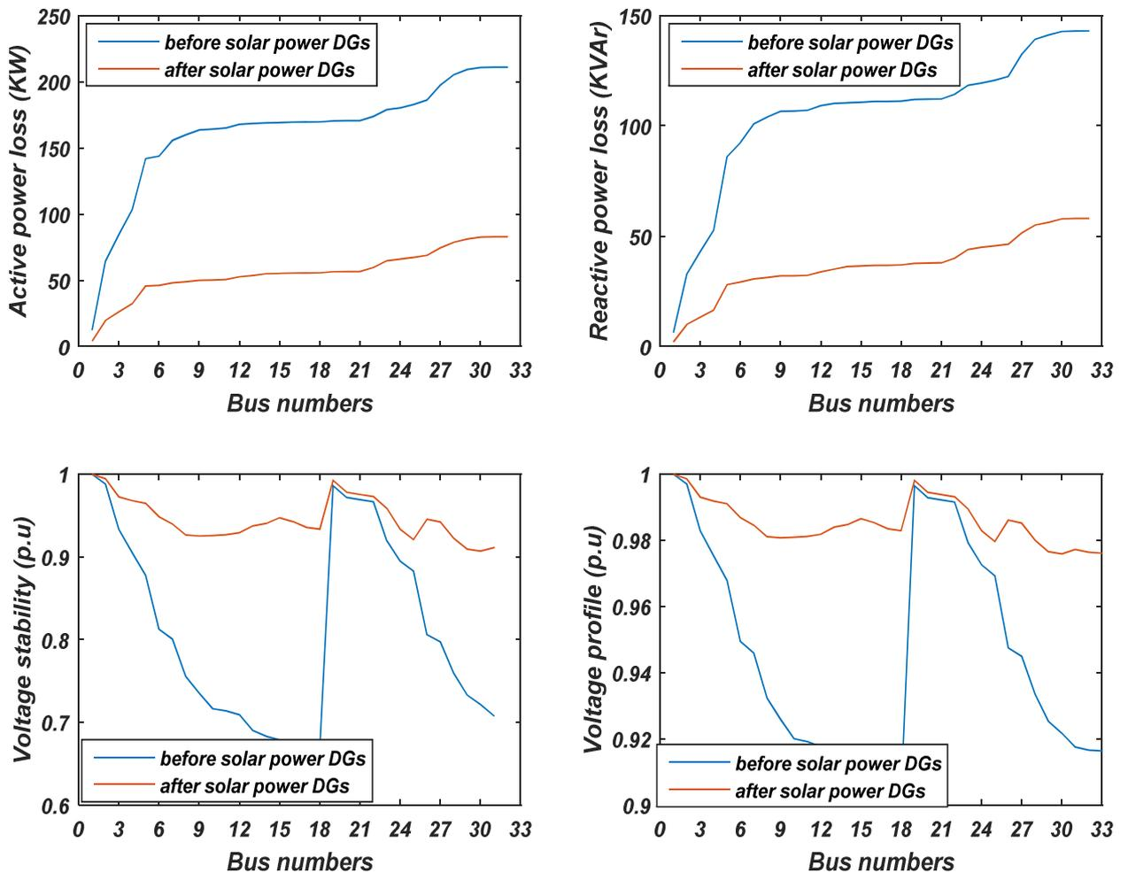
Figure 5. Power losses, voltage stability and voltage profile of each bus/branch before and after installation of solar power DG.
