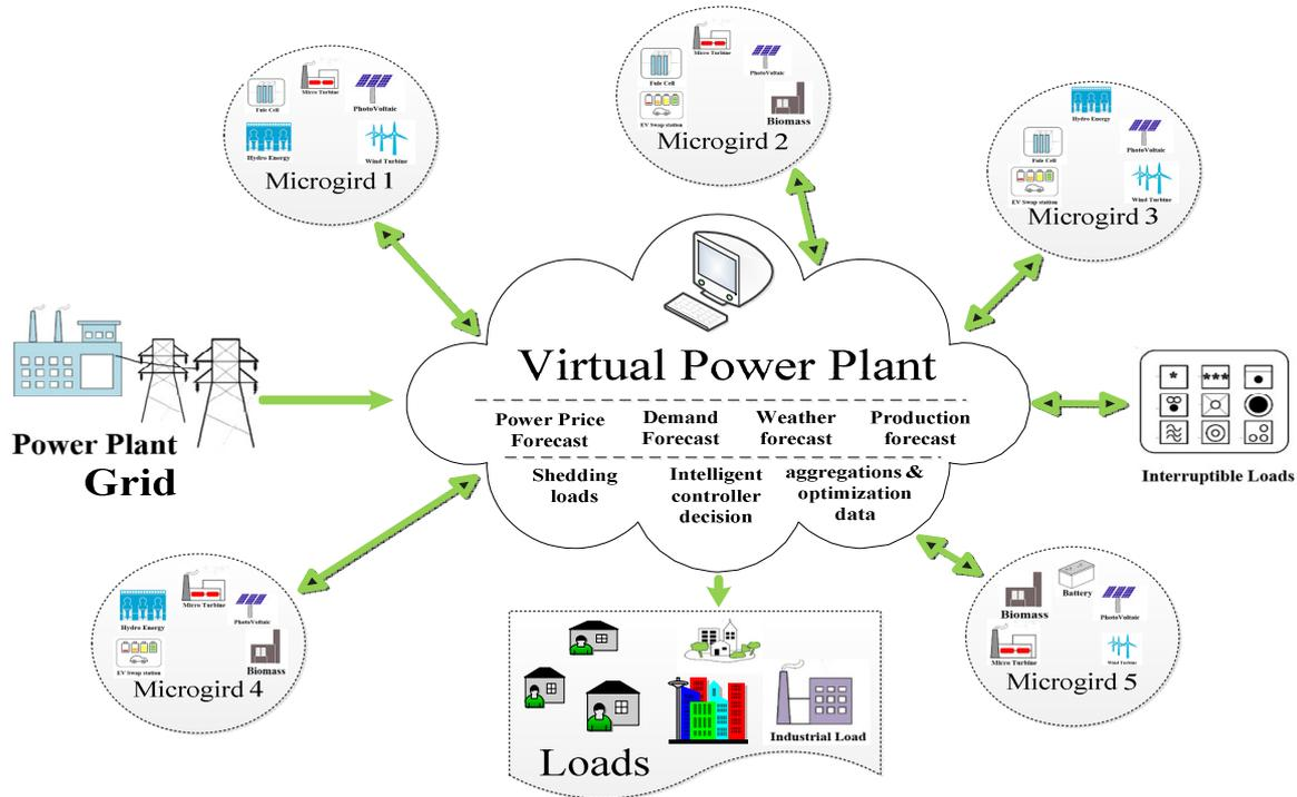
Fig. 1 Virtual power plant and Microgrids including distributed generators.
