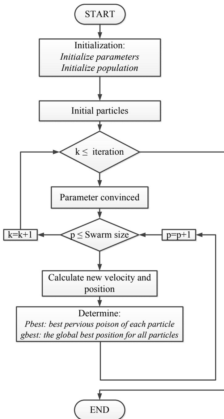
Fig.4. Flow chart for PSO algorithm.
