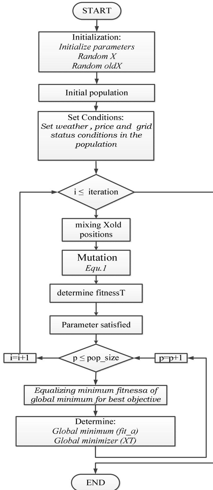
Fig.3 BSA algorithm flowchart.
