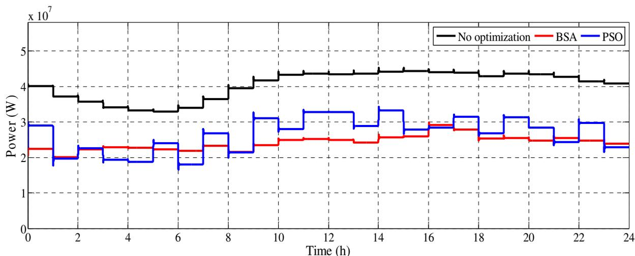
Fig.8. Distribution substation power comparison without optimisation, with BSA and PSO.
