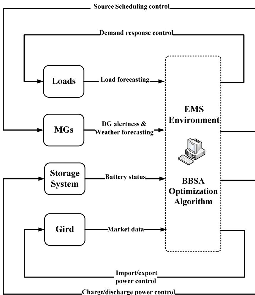
Fig.2 EMS based on an algorithm input and output control flow
