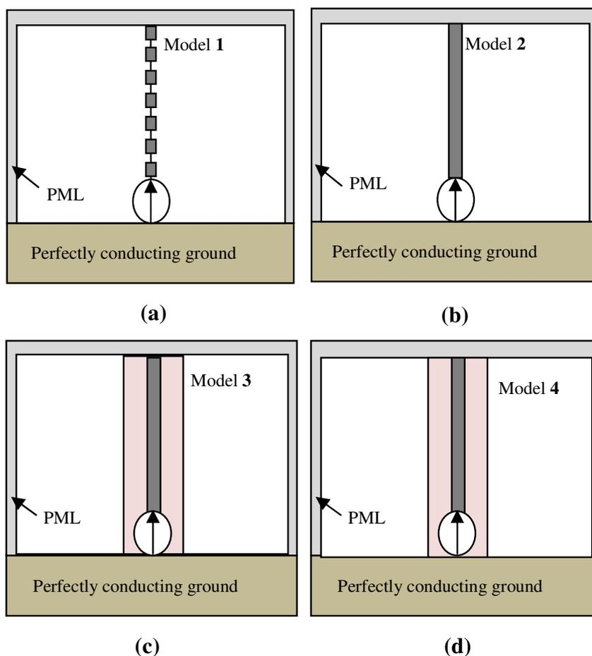
Fig. 1. Two lightning return stroke channel representations with a perfectly conducting ground excited at its bottom by a current source:
