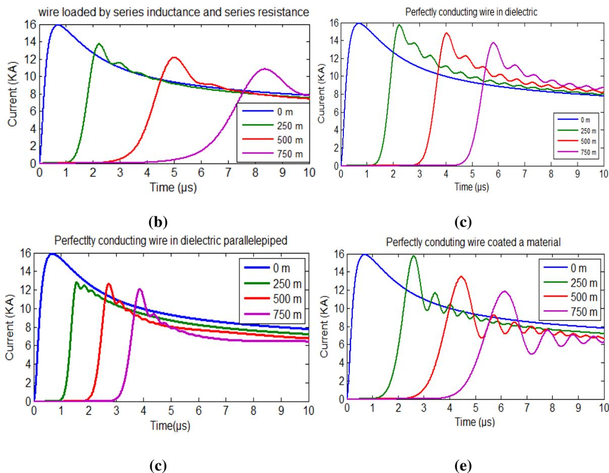
Fig. 2 Current waveforms calculated at different heights using the 3D-FDTD method and EM models:
