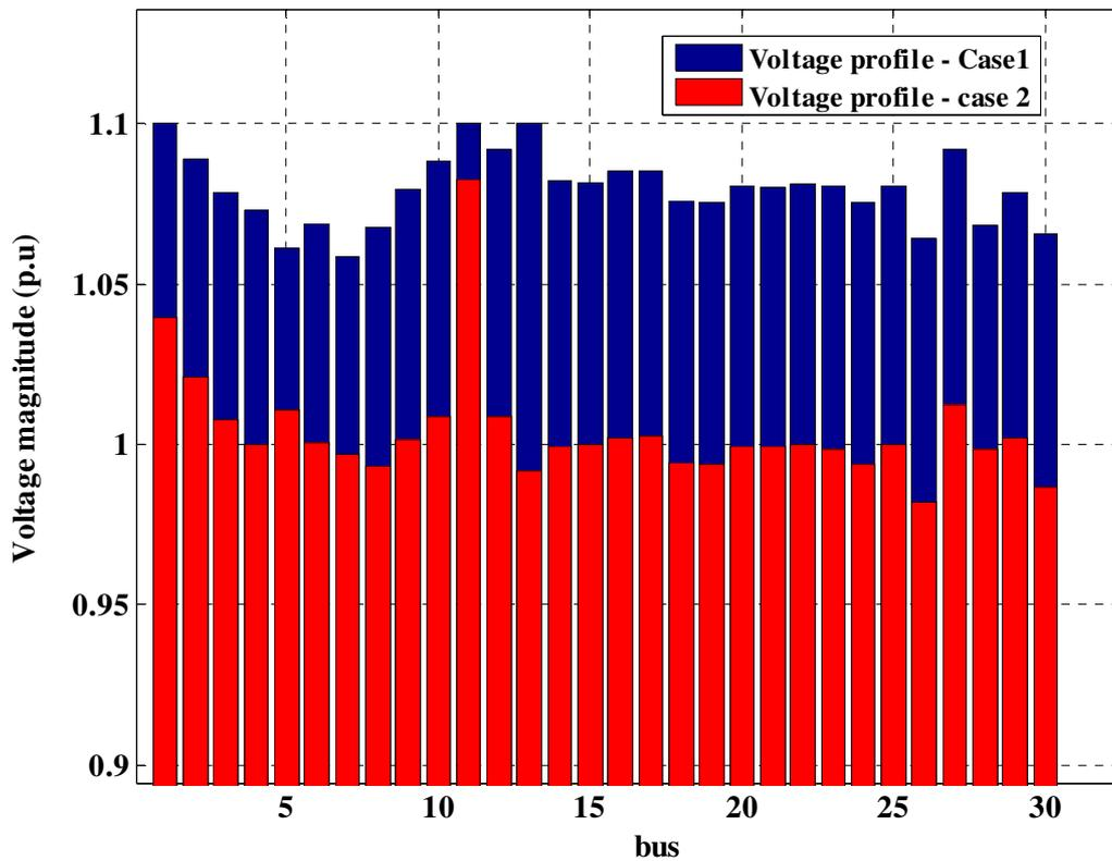
Fig. 3 Voltage profile for both cases 1 and 2 – IEEE30 bus test system
