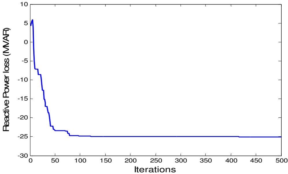
**Figure.6** Variations of reactive power transmission losses for Case 5.
