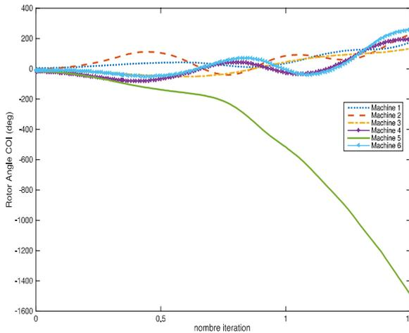
Fig.7. Rotor angle curves with IPSO solution for IEEE 30-bus system
