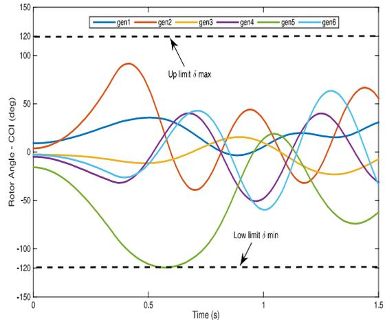
Fig.8. Rotor angle curves with TSCOPF solution case
