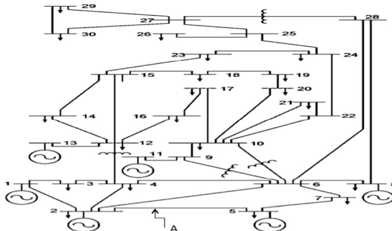
Fig.6. Single-line diagram of IEEE 30-bus system
