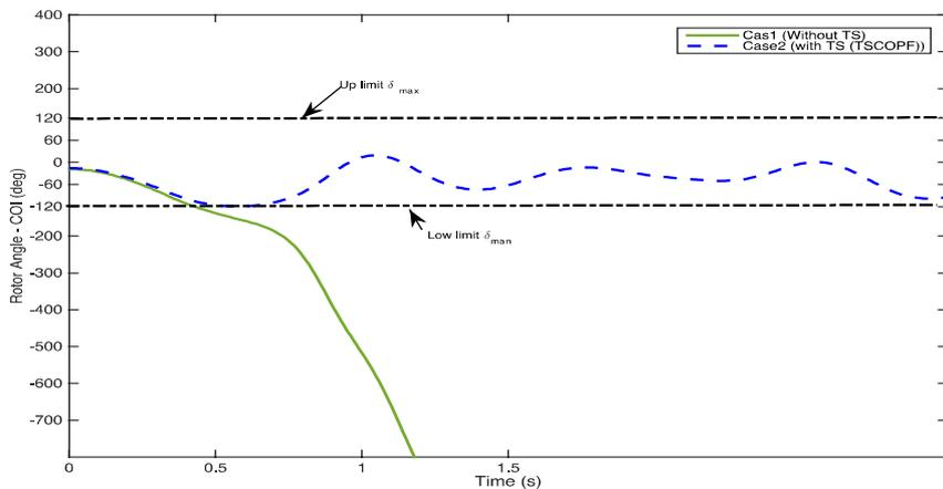
Fig.9. Rotor angle curves for the 5<sup>th</sup> generator with IPSO and TSCOPF solutions.
