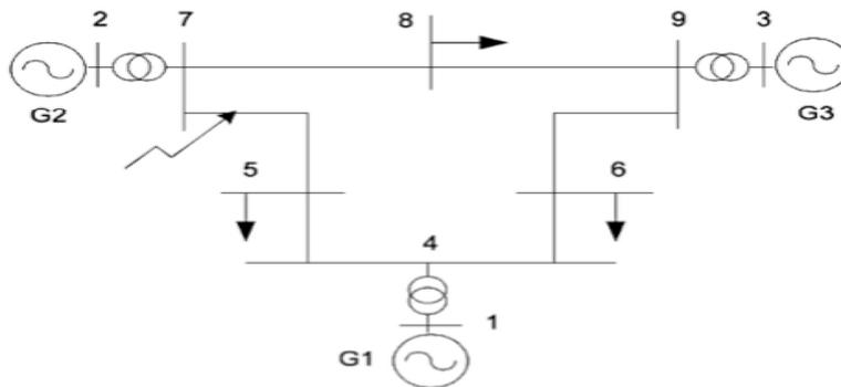
Fig.3. WSCC 3-machine 9-bus test system
