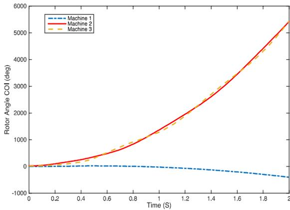
Fig. 4. Rotor angle curves based after OPF solution in WSCC 9-bus system.
