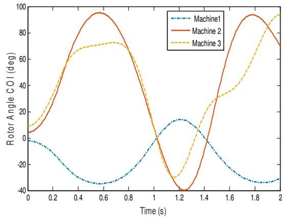
Fig. 5. Rotor angle curves based after TSCOPF solution in WSCC 9-bus system.
