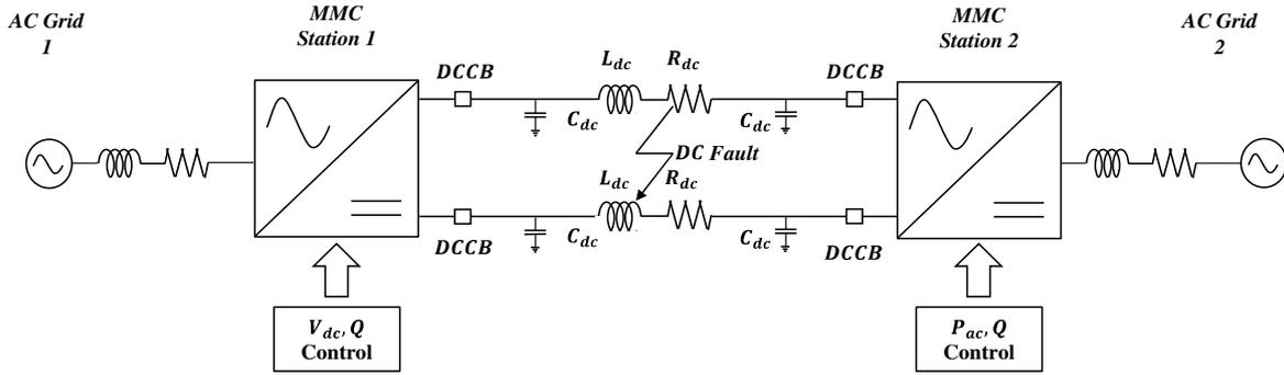
Fig. 7. Simulation circuit for fault condition
