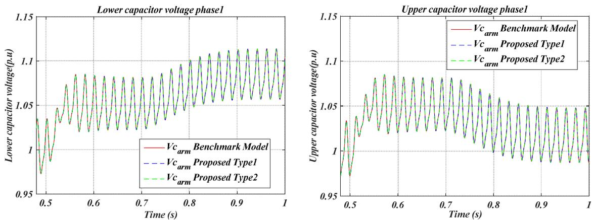
Fig. 6. MMC 1: Lower capacitor voltages (Left), Upper capacitor voltages (Right)
