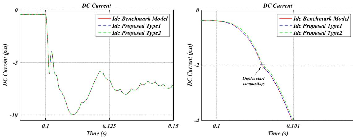
Fig. 8. DC current variation in MMC 1 (Left), Zoom on DC current fault (Right)
