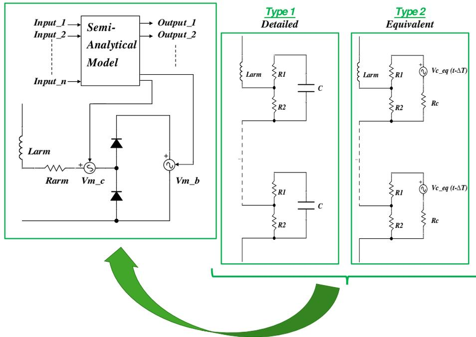
Fig. 3. Proposed MMC model for full order MMC types
