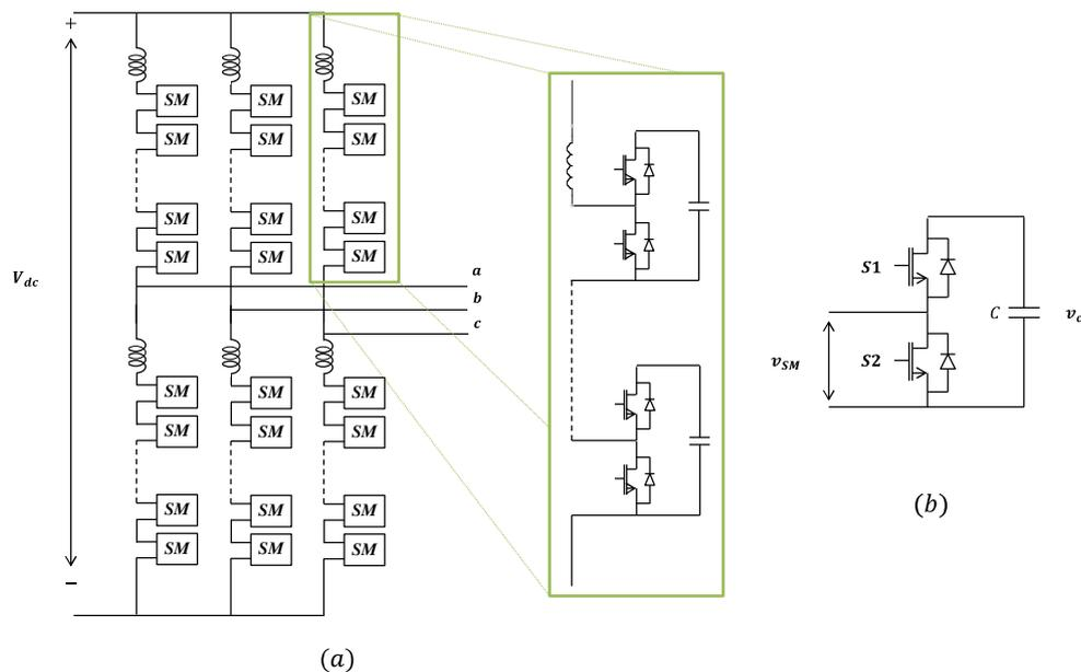
Fig. 1. (a) Three-phase half bridge MMC topology, (b) Half bridge submodule
