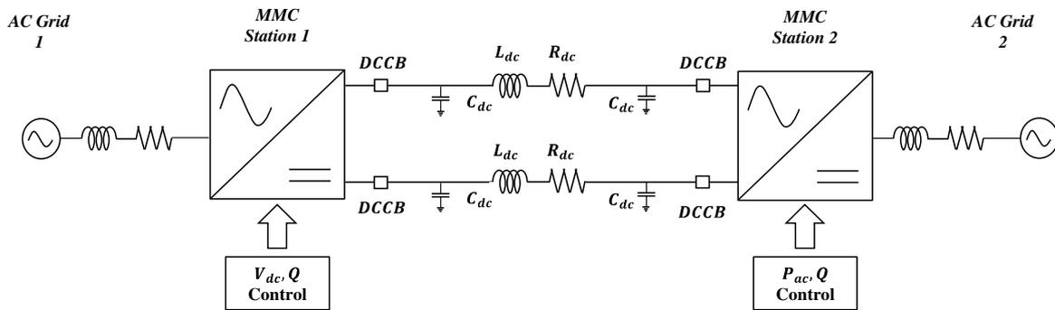
Fig. 4. Simulation circuit
