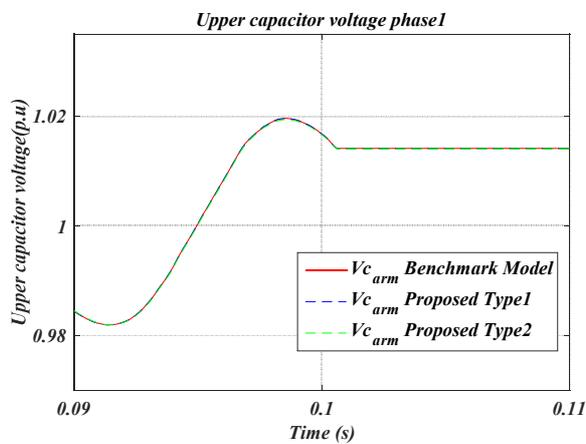
Fig. 8. Upper capacitor voltages in MMC 1 for DC fault condition
