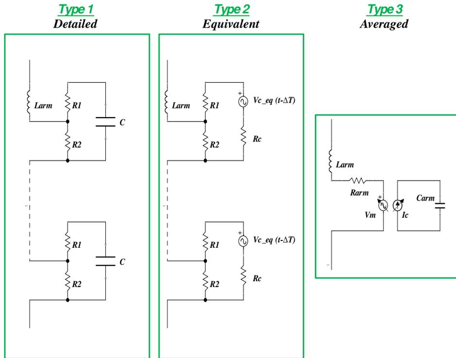
Fig. 2. Different MMC arm models presented in literature: Type1, Type 2 and Type 3
